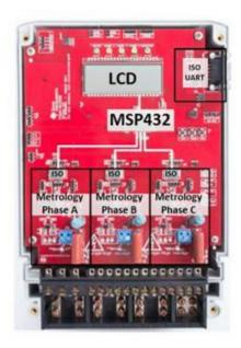
Figure 1. Setup for a smart meter with an MSP432 MCU
