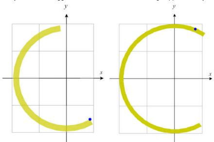
Figure 5-1. Magnet Position Trace Due to Installation Error
