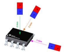
Figure 3-1. 3D Hall Sensor Axis
