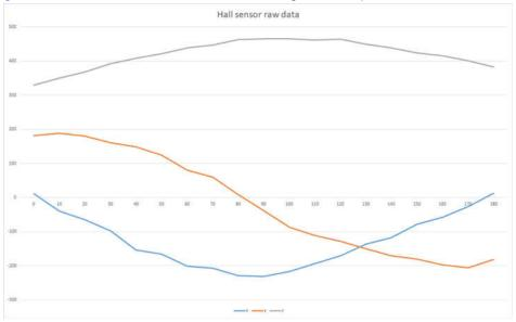
Figure 5-2. Hall Sensor Output Raw Data From 0° Through Approximately 180° of Collision
