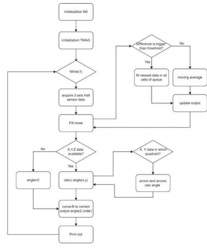
Figure 6-2. Firmware Flowchart
