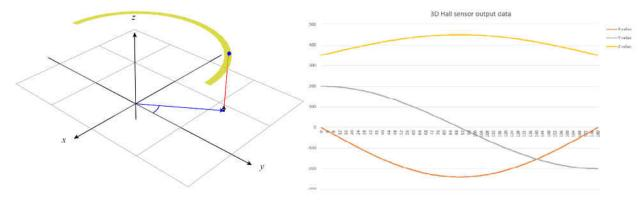
Figure 4-3. Angle Calculation and Output Data Waveform of Hall Sensor
