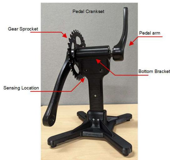
**Figure 2-1. Gear Tooth Sensing Setup**
