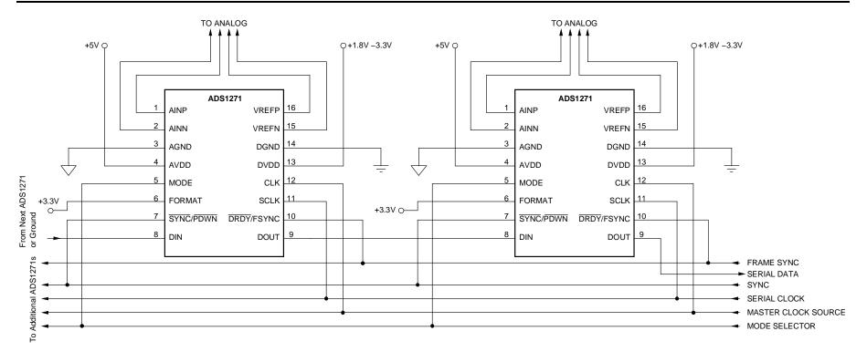
Figure 2. Simultaneous Sampling in FSYNC Mode
