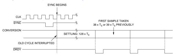
Figure 3. Synchronization Timing
