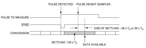
Figure 4. Synchronizing the ADS1271 to a Pulse
