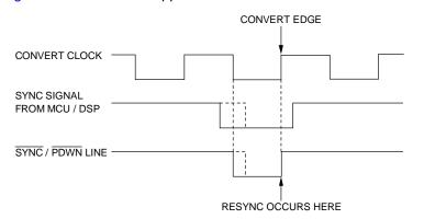
Figure 6. Resynchronization Timing
