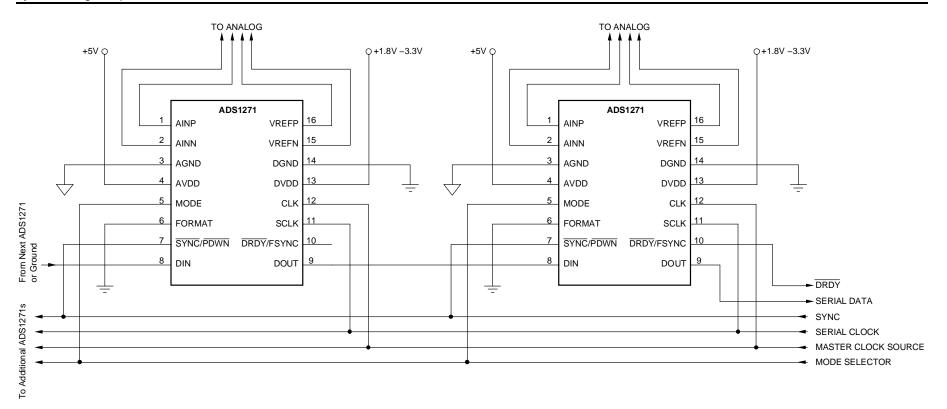
Figure 1. Simultaneous Sampling in SPI Mode
