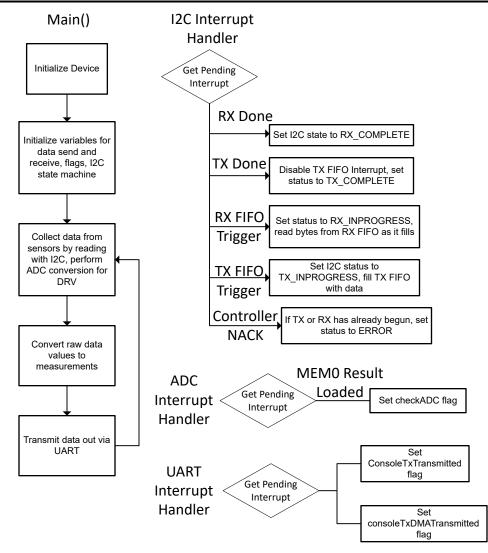
Figure 1-2. Application Software Flowchart
