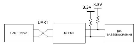
Figure 1-1. System Functional Block Diagram
