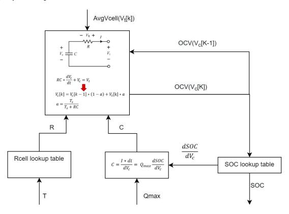
Figure 3-3. VGauge Software Flow
