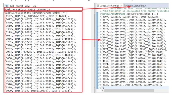
Figure 4-4. Battery Circuit Table Input
