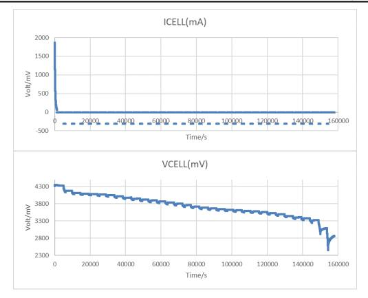
Figure 4-1. Pulse Discharge Test Case
