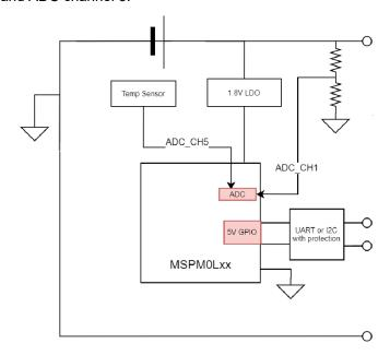
Figure 2-1. MSPM0 Gauge Board Block Diagram
