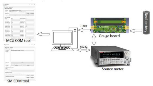
Figure 4-2. Hardware Structure to Get Battery Model
