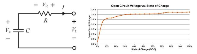
Figure 3-2. Battery Model and SoC-OCV Table
