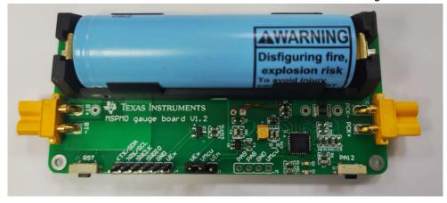
Figure 1-1. MSPM0 Gauge Hardware Board
