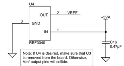
Note: If U4 is desired, make sure that U3 is removed from the board. Otherwise, Vref output pins will collide.
