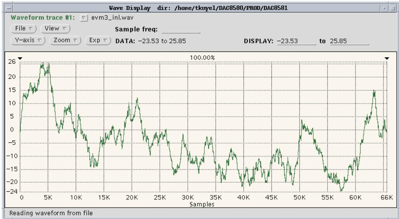
**Figure 8. INL Characteristic Plot for the DAC8581**
