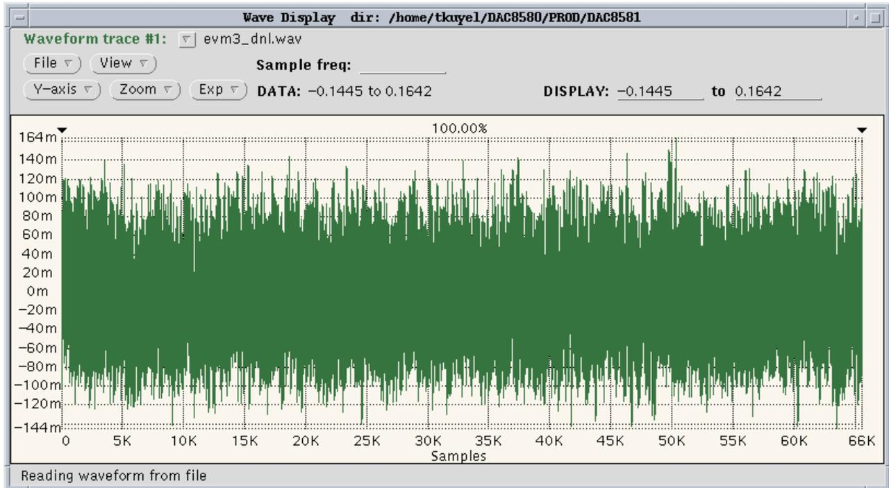
**Figure 9. DNL Characteristic Plot for the DAC8581**
