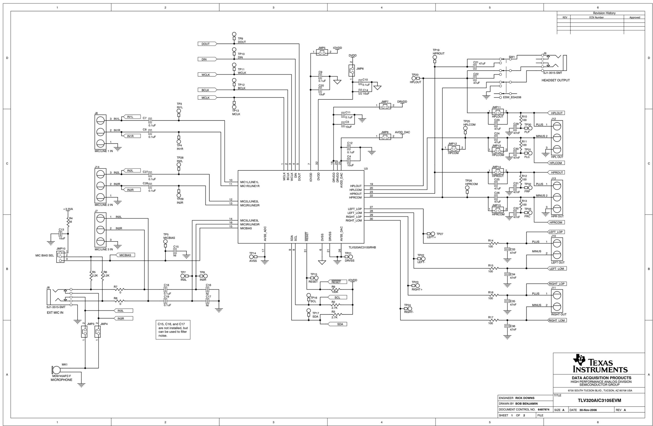
C15, C16, and C17 are not installed, but can be used to filter noise.
