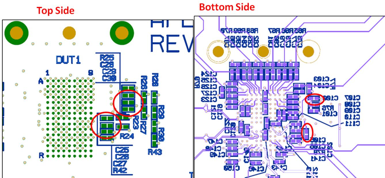
**Figure 22. Relevant Capacitors for CW Mode, Top and Bottom Side**
