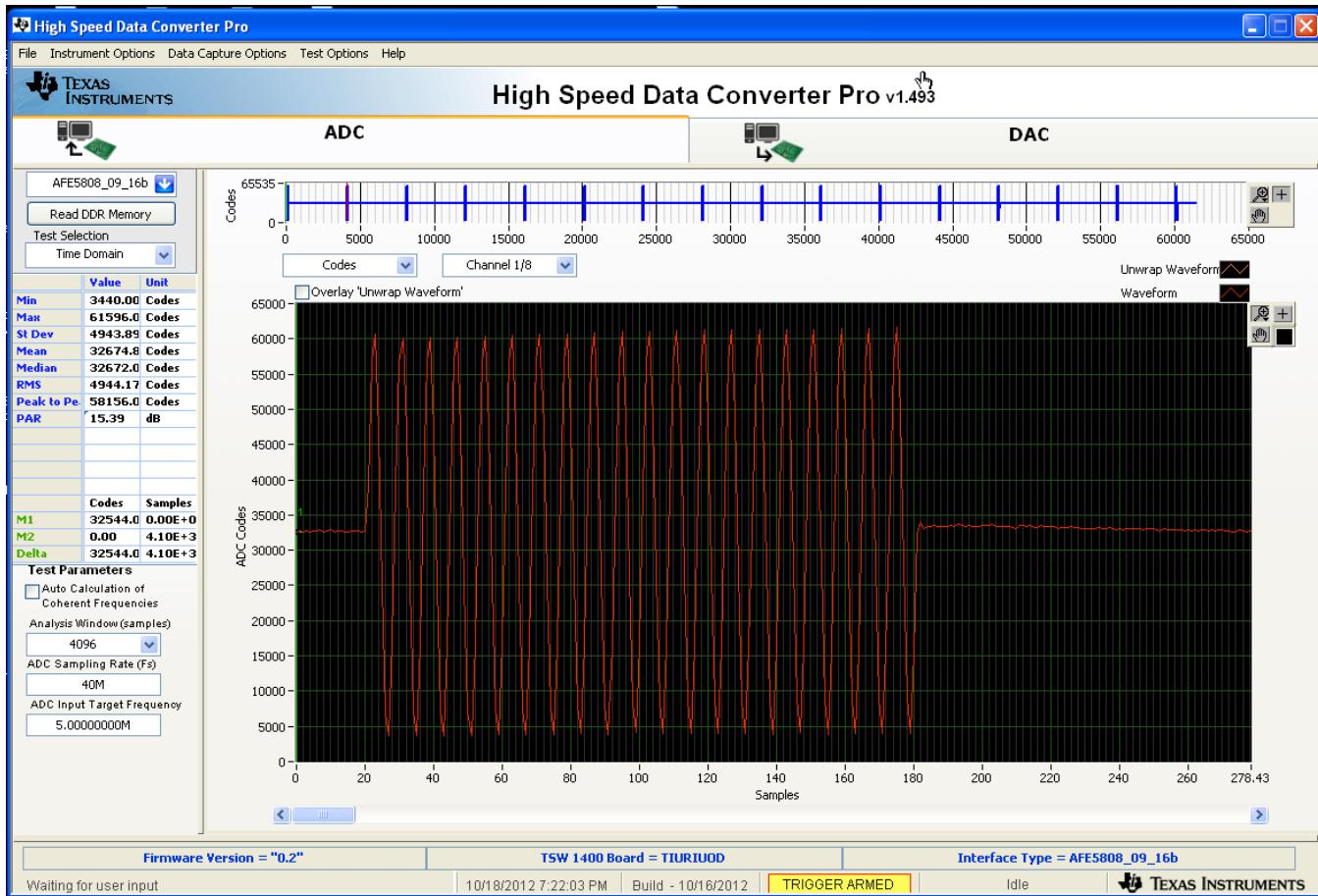
Figure 11. Analog Sine Burst with 20 Cycles at 10 MHz
