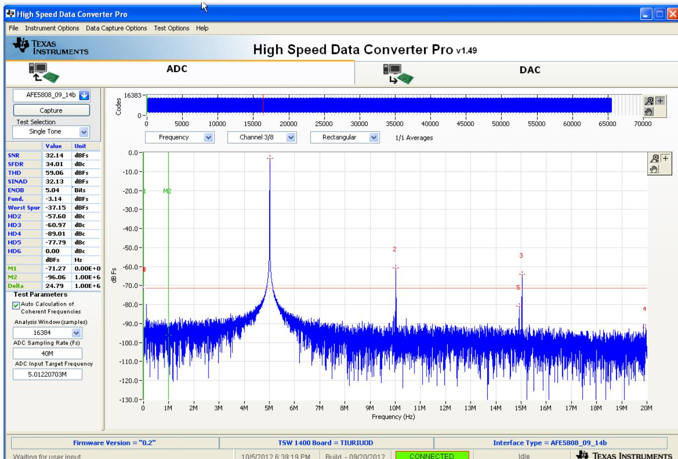
**Figure 24. GUI Screen for Windowing Option Selection**
