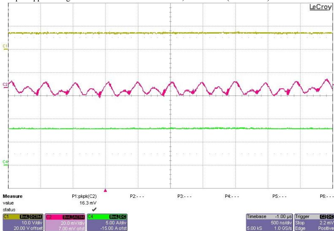
The output ripple voltage is shown in the figure below with Vin=7.2V, Iout = 12A. (20mV/DIV)
