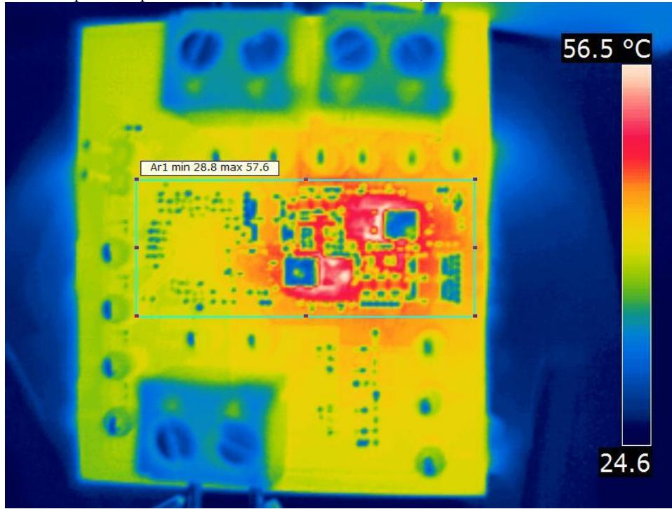
The converter temperature profile is shown below at Vin = 7.5V, Iout= 12A.
