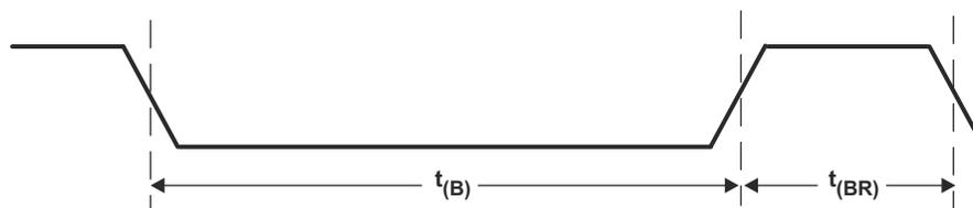
**Figure 9-2. HDQ Break and Break Recovery Timing**
