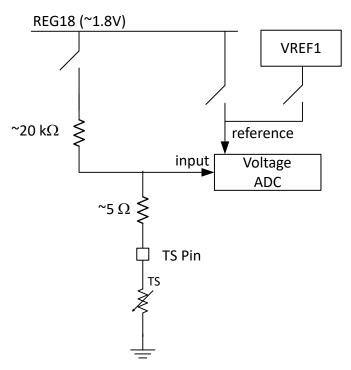
Figure 7-1. BQ76905 TS Pin Configuration
