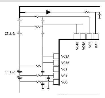
Figure 5-1. Connecting an Unused Cell Input Pin
