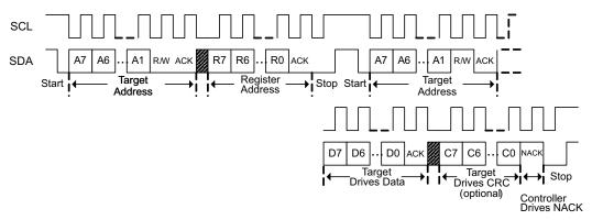
Figure 9-3. I<sup>2</sup>C Read without Repeated Start
