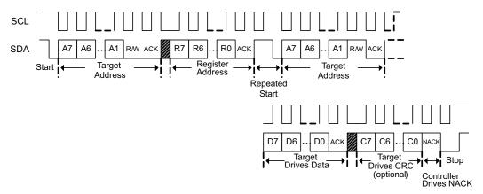
Figure 9-2. I<sup>2</sup>C Read with Repeated Start
