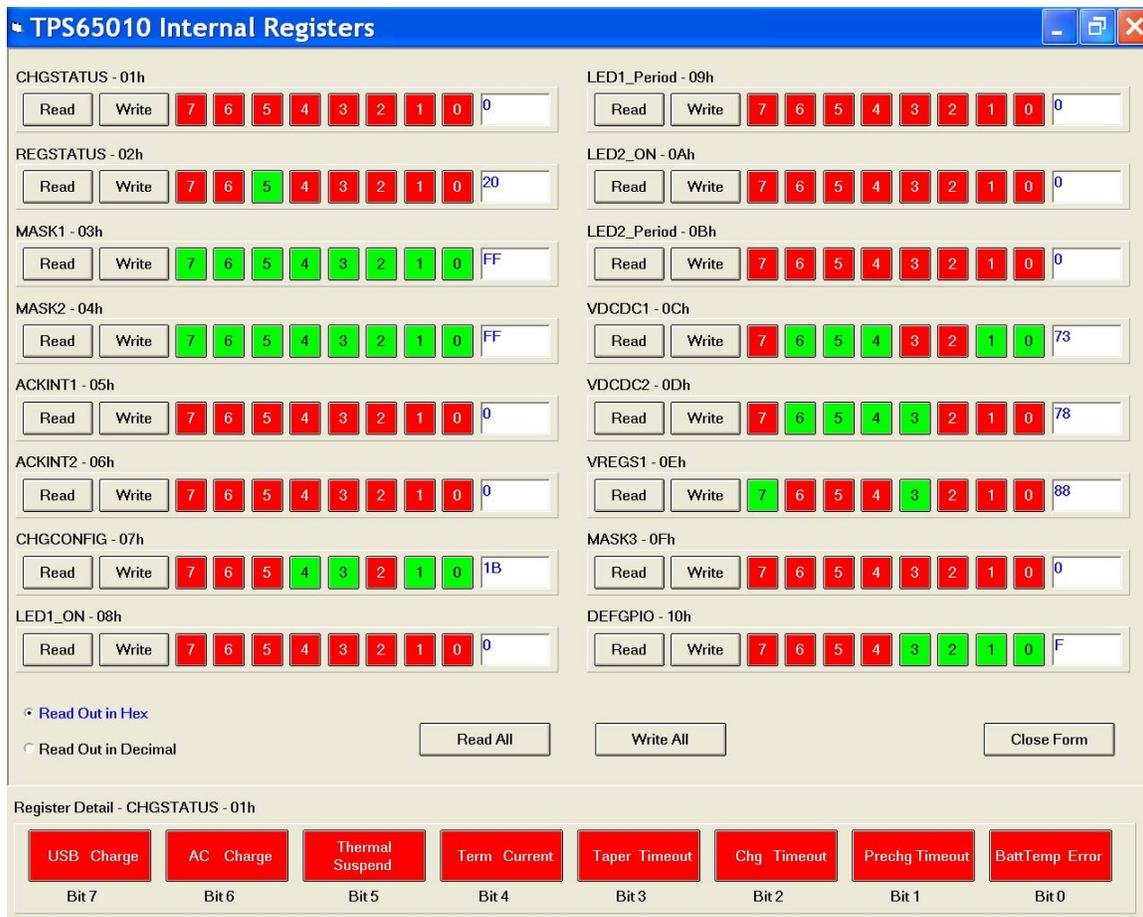
Figure 2. Internal Registers Window
