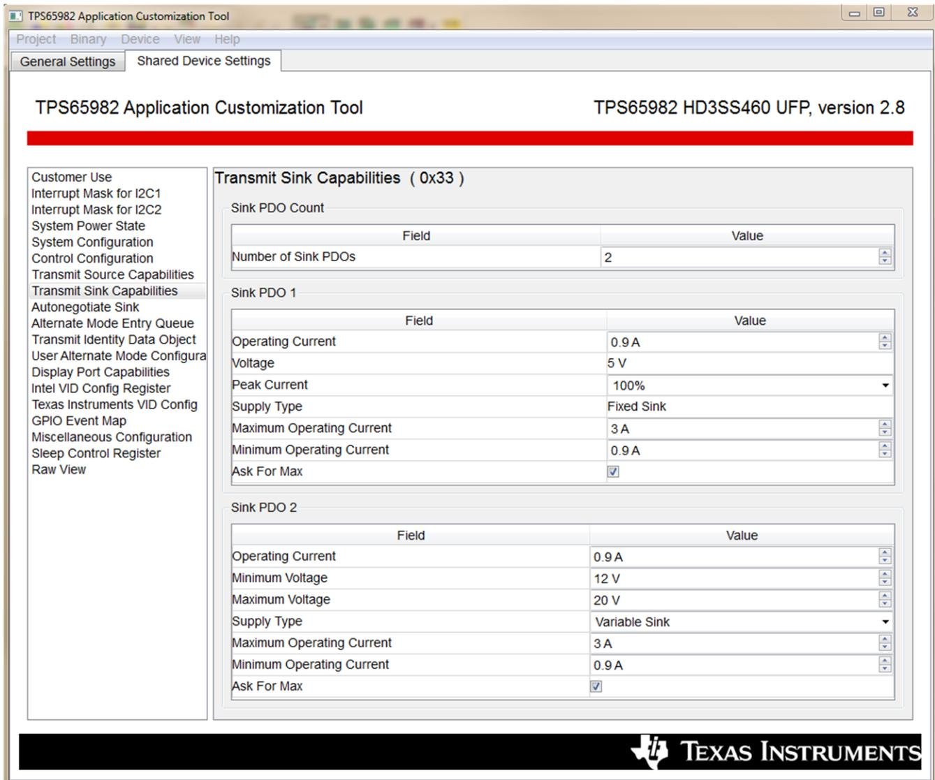
Figure 3. Tx Sink Capabilities Register of *TPS65982\_HD3SS460\_UFP\_Full\_2\_8.tpl*
