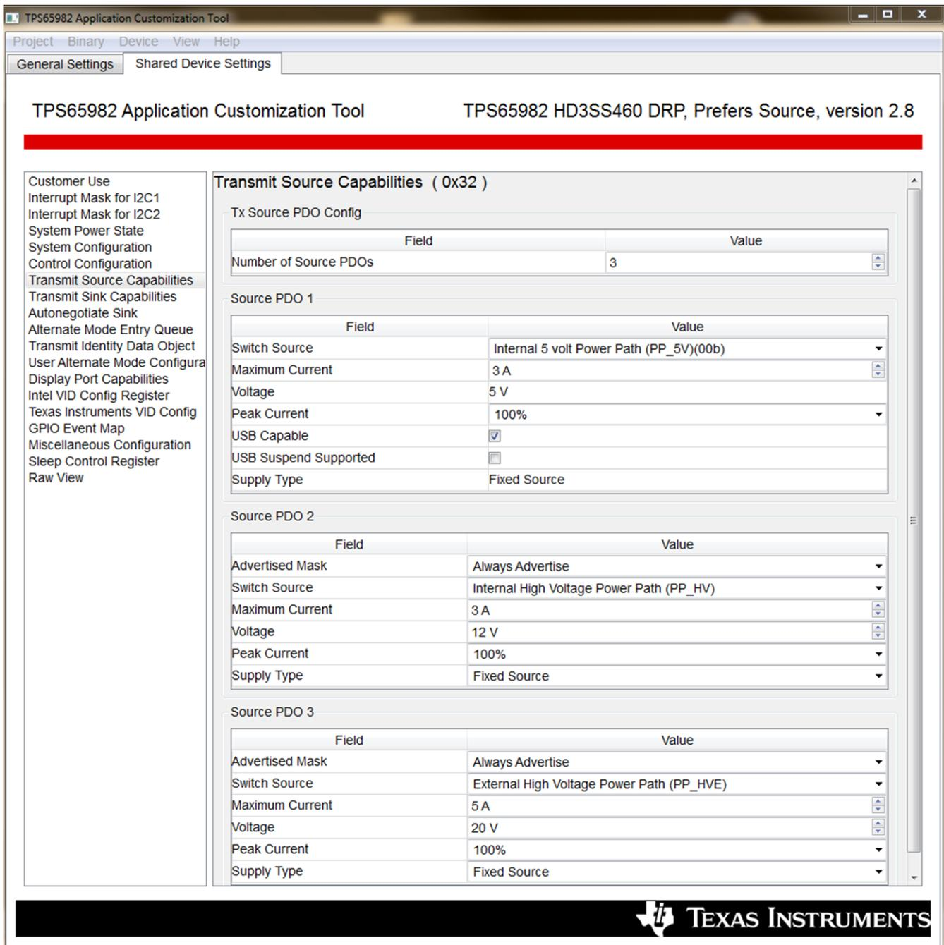
Figure 1. Tx Source Capabilities Register of *TPS65982\_HD3SS460\_DRP\_Source\_Full\_2\_8.tpl*
