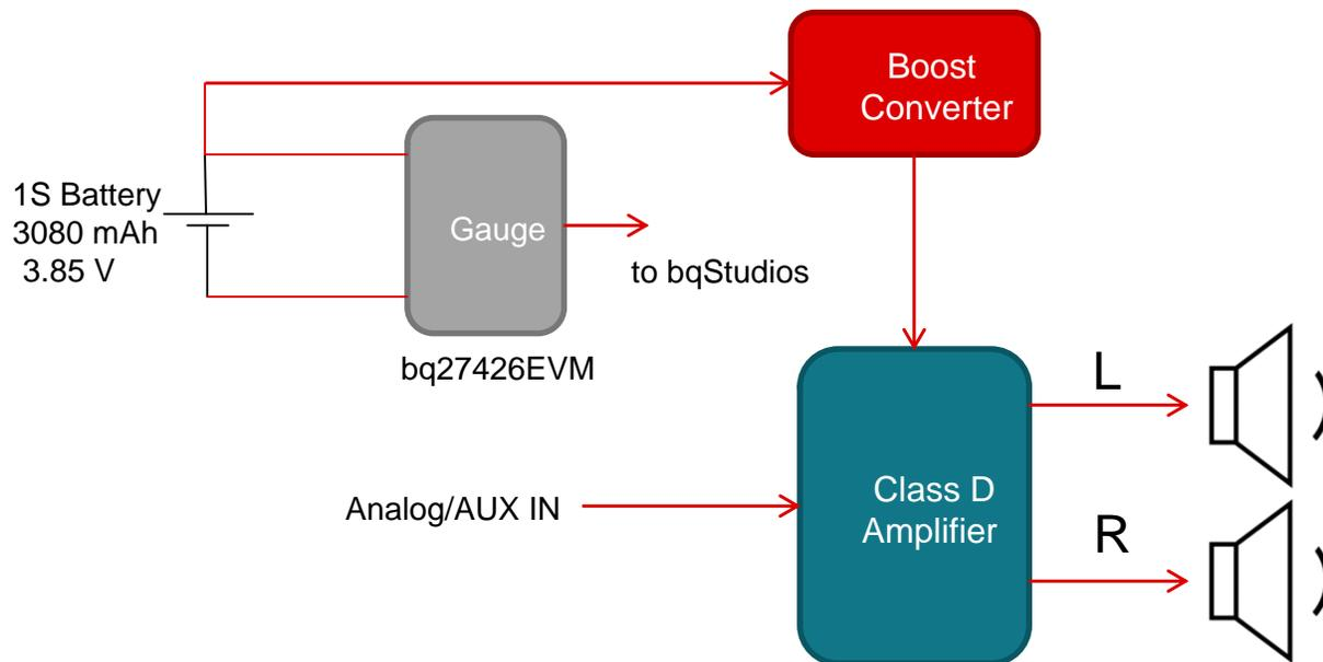
**Figure 1. Setup Block Diagram**
