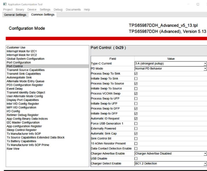
**Figure 3. Port Control Register (0x29) Advanced Settings Tab for "Preferred Host"**
