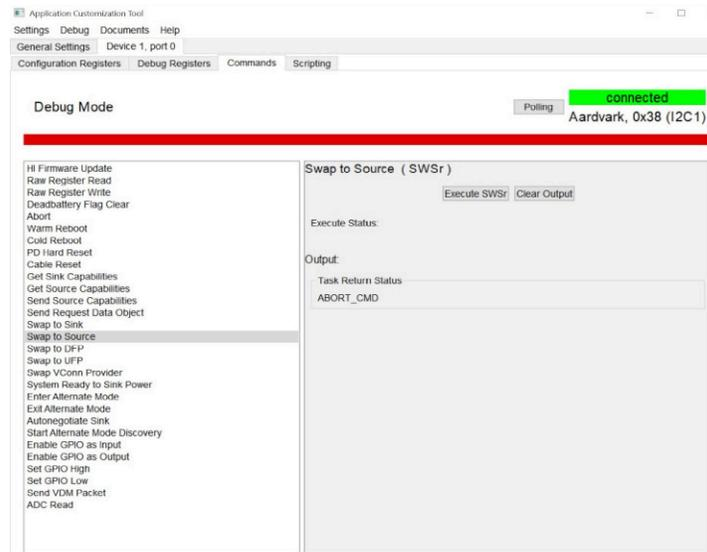
**Figure 8. Failed SWSr When Dead Battery flag is Set to 1 (True)**
