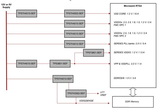
Figure 4-2. Rad-Tolerant Power for RTG4
