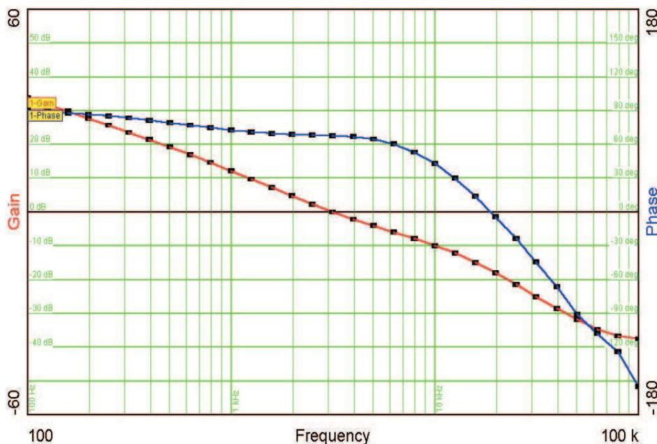
**Figure 9. Loop Gain of the Flyback Converter With 48-V Input and 2-A Load**
