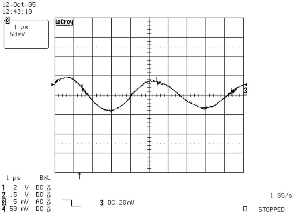
Figure 3. Input Voltage Ripple and Noise Measured at J4 With 48V Input and Max Load on Output
