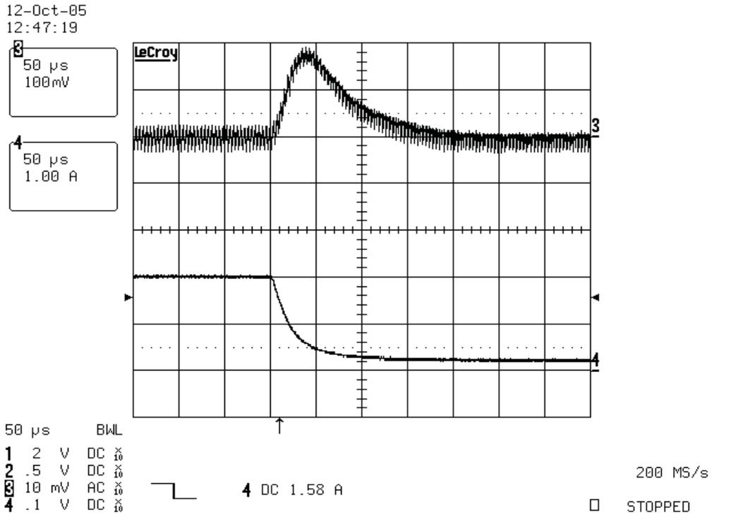
Figure 5. The Output Voltage Transient Response With a Load Step From 90% to 10%
