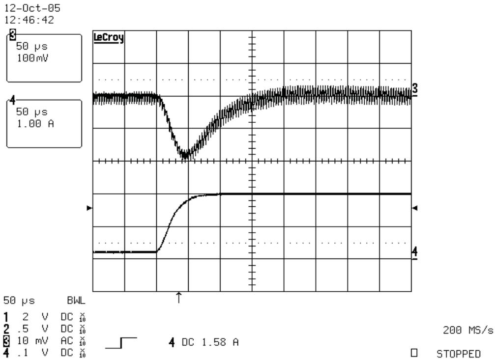
Figure 4. The Output Voltage Transient Response With a Load Step From 10% to 90%
