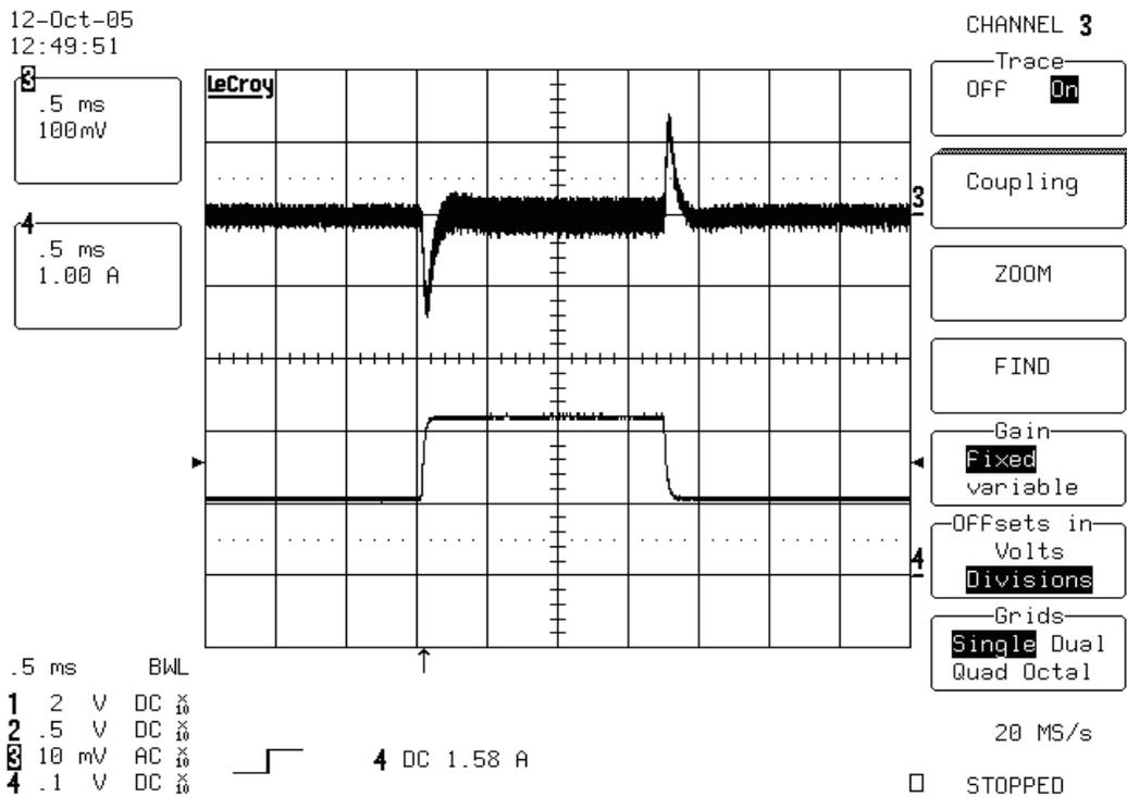
Figure 6. The Output Voltage Transient Response With a Load Step From 50% to 100%
