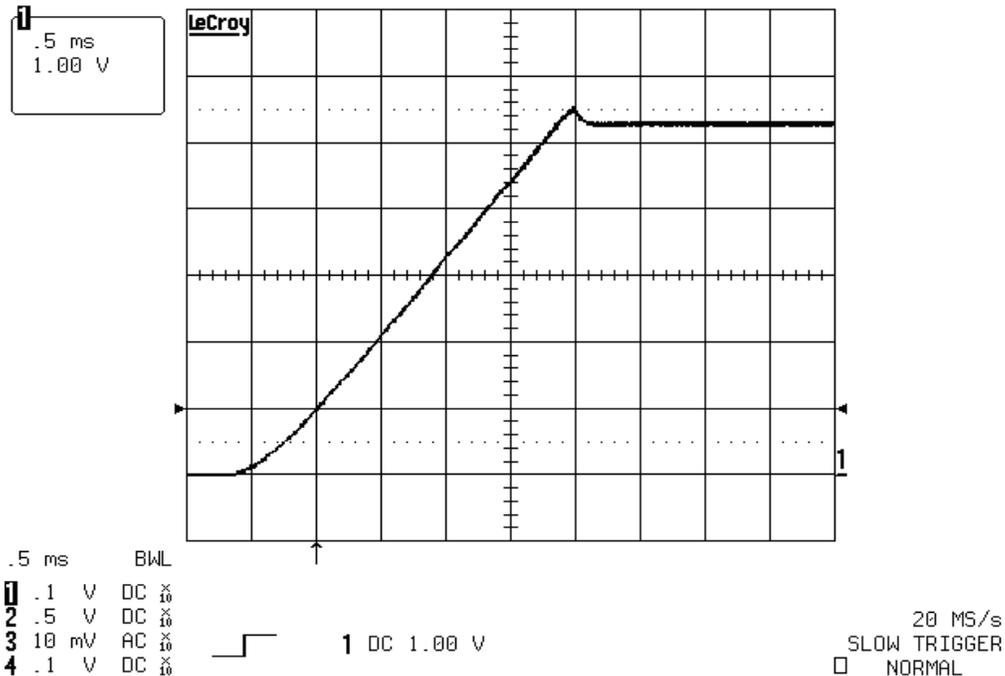
Figure 7. The Output Voltage Turn-On Response With a 48V Input and a 2A Load
