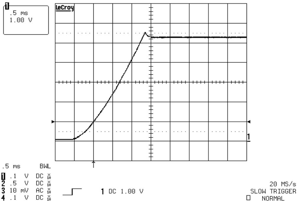
Figure 8. The Output Voltage Turn-On Response With a 48V Input and a 0A Load
