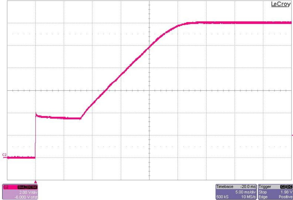
The photo below shows the output voltage startup waveform after the application of 3.8V in. The 12V output was loaded to 4A. (2V/DIV, 5mS/DIV)
