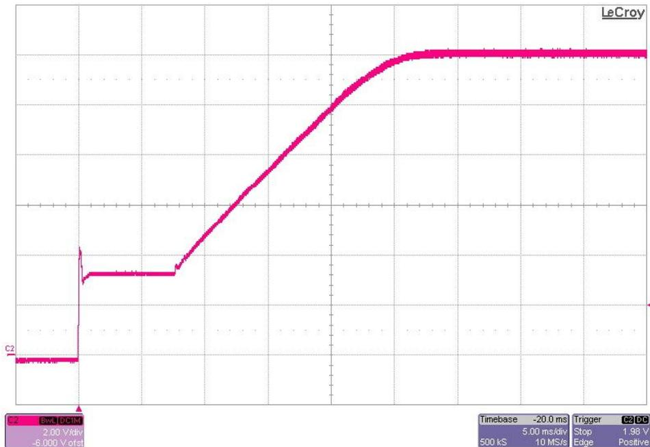
The photo below shows the output voltage startup waveform after the application of 7.6V in. The 12V output was loaded to 0A. (2V/DIV, 5mS/DIV)
