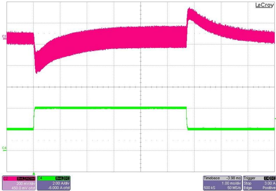
The photo below shows the output voltage (ac coupled) when the load current is stepped between 2A and 4A.  $V_{in} = 7.6V$ . (100mV/DIV, 2A/DIV, 1mS/DIV)
