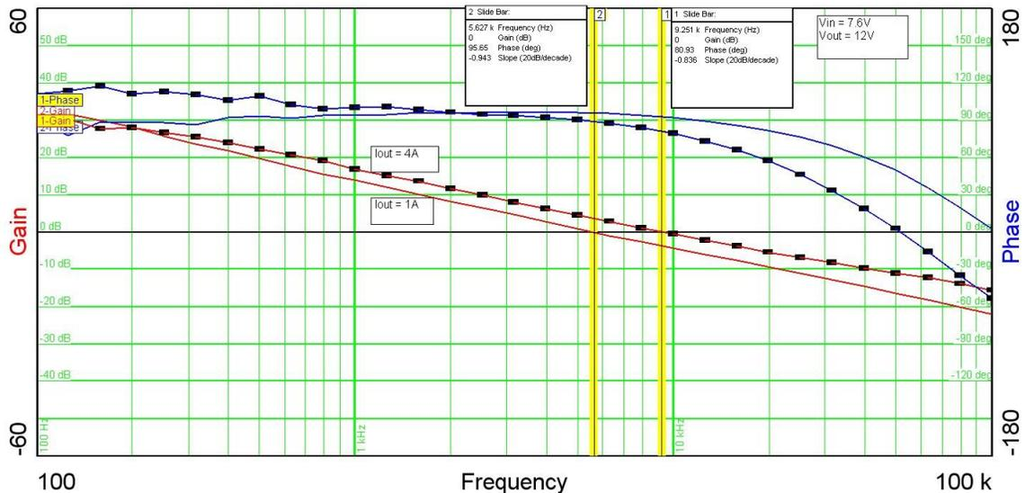
The plot below shows the loop gain and phase margin with the output loaded to 1A and 4A. The input voltage was set to 3.8V.
