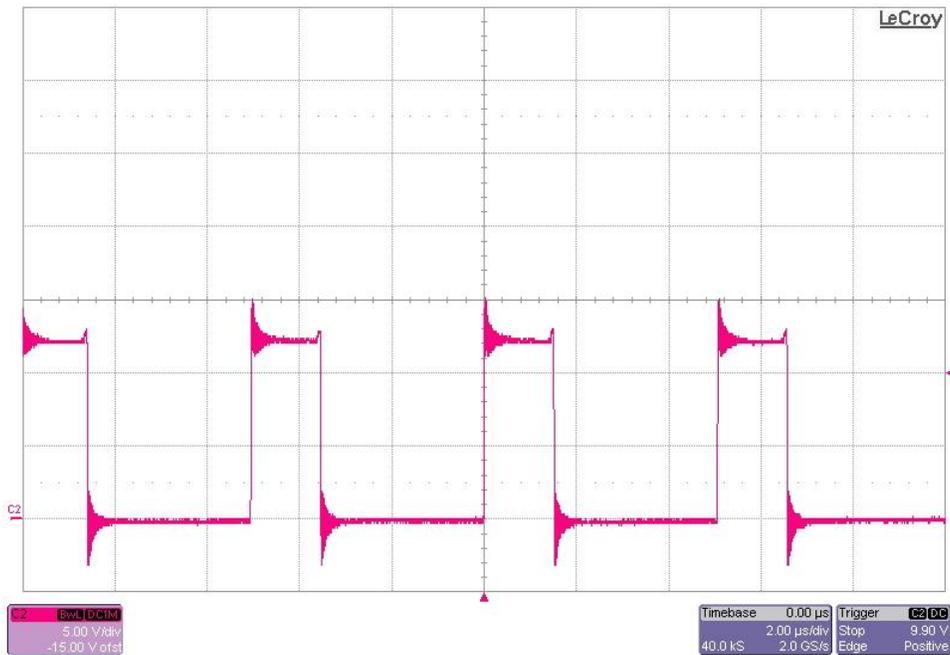
The photo below shows the FET switching voltage. The input voltage is 7.6V and the output is loaded to 4A. (5V/DIV, 2uS/DIV)
