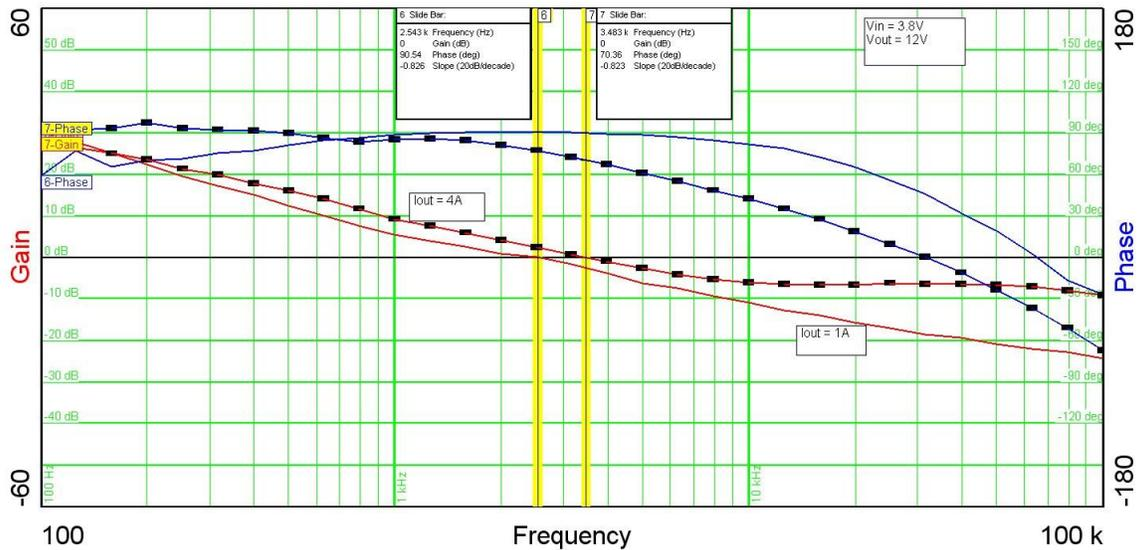
The plot below shows the loop gain and phase margin with the output loaded to 1A and 4A. The input voltage was set to 3.0V.
