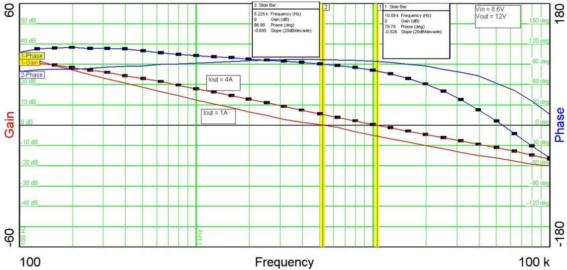
The plot below shows the loop gain and phase margin with the output loaded to 1A and 4A. The input voltage was set to 7.6V.
