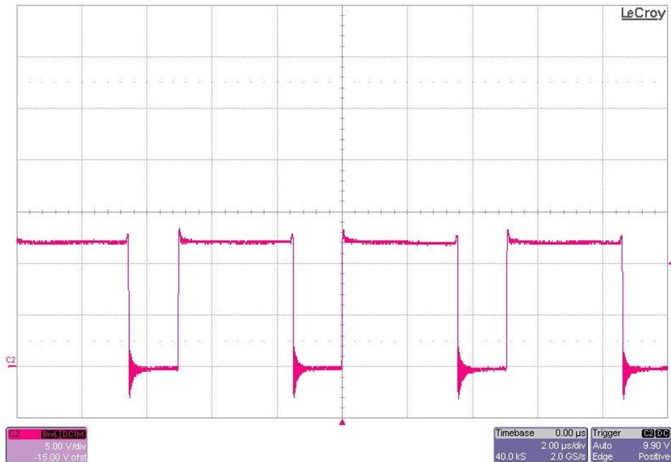
The photo below shows the FET switching voltage. The input voltage is 3.8V and the output is loaded to 0.4A. The boost converter is starting discontinuous mode operation. (5V/DIV, 2uS/DIV)
