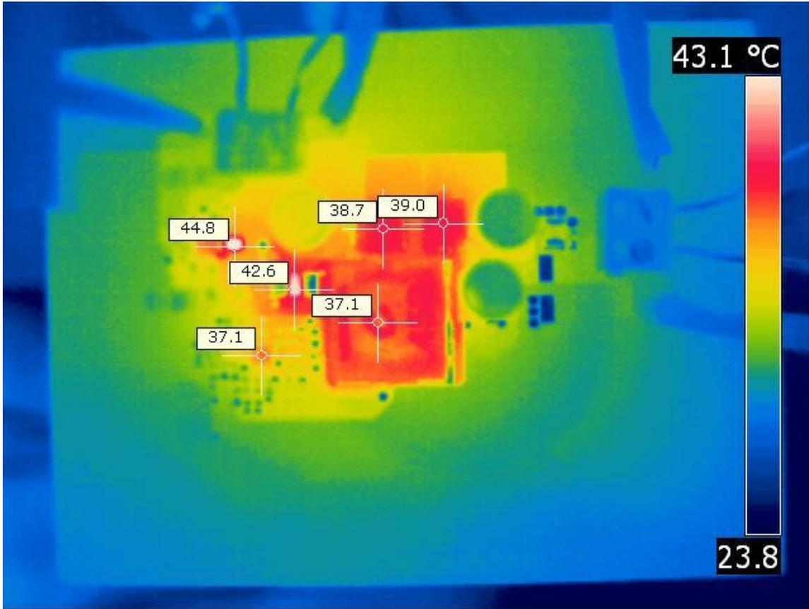
A thermal image is shown below operating at 3.8V input and 4A output (room temp and no airflow).
