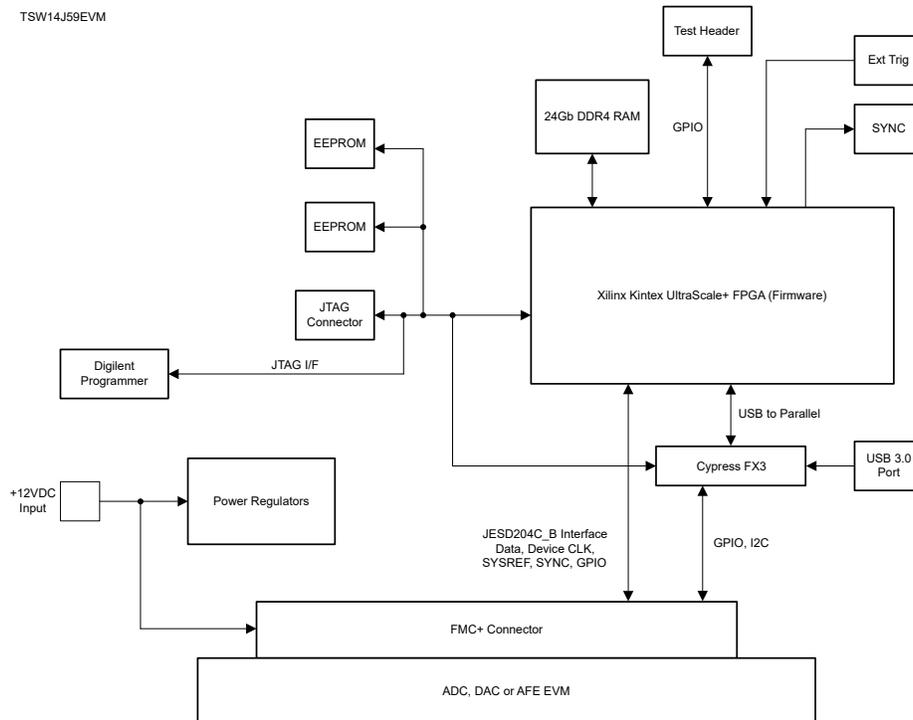
**Figure 2-2. TSW14J59EVM Block Diagram**
