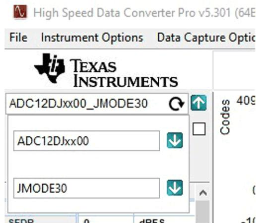
Figure 5-4. Example When Connected to an ADC12DJ3200EVM Using JMODE30
