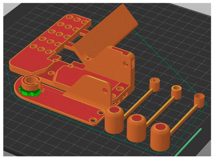
Figure 3-12. Part Orientation in Slicer
