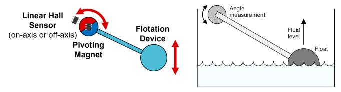
Figure 2-8. Pivoting Magnet Float Arm Implementation
