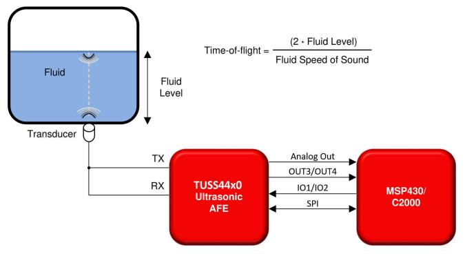
Figure 2-2. Ultrasonic Liquid Level Sensing
