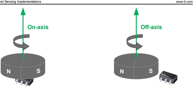
Figure 2-9. On-Axis vs. Off-Axis Angle Measurements
