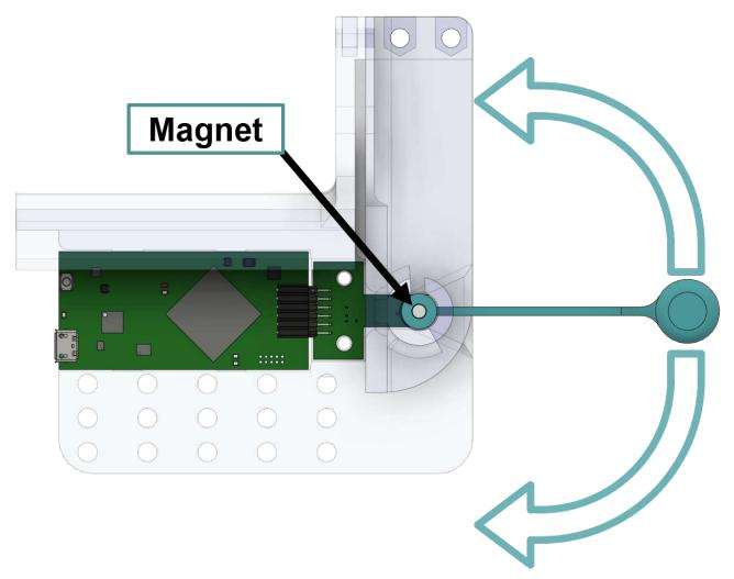
Figure 3-5. Float Rotation and Magnet Placement
