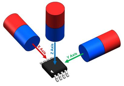
Figure 2-3. 3D Hall Sensor Axis
