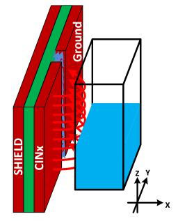
Figure 2-1. Capacitive Liquid Level Sensing
