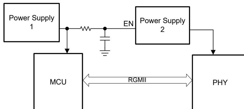
Figure 4. RC Delay-Based Solution
