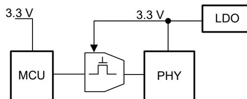
Figure 3. Switch-Based Solution
