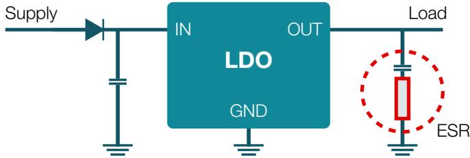
**Figure 29:** Output capacitor and ESR.
