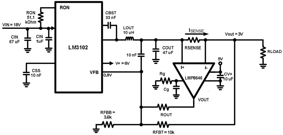
Figure 5 – Recommended Components for the LM3102
