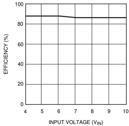
**Figure 3-3. Efficiency vs Input Voltage ( $I_{out} = 2\text{ A}$ )**
