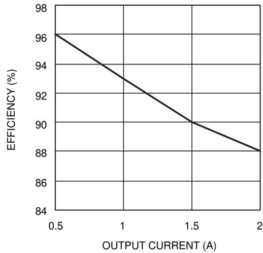
**Figure 3-2. Efficiency vs Output Current ( $V_{IN} = 5\text{ V}$ )**
