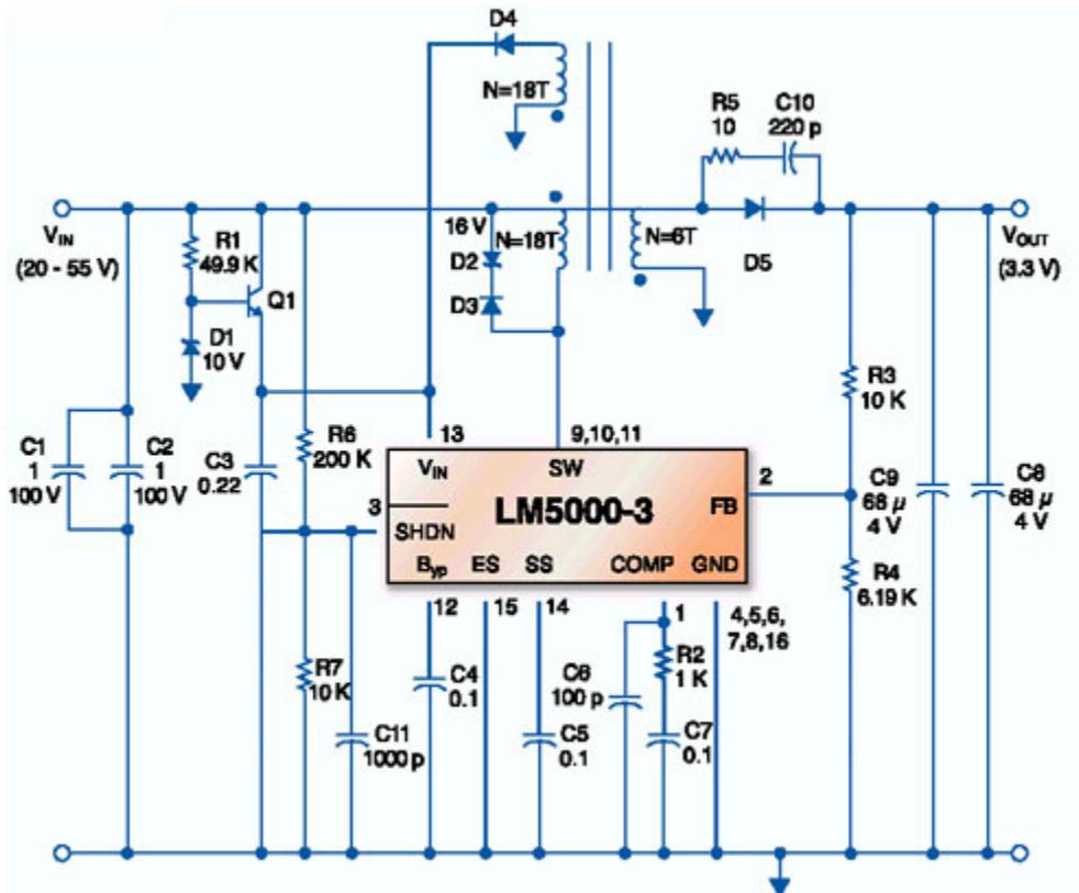
Figure 1. LM5000 Flyback Converter
