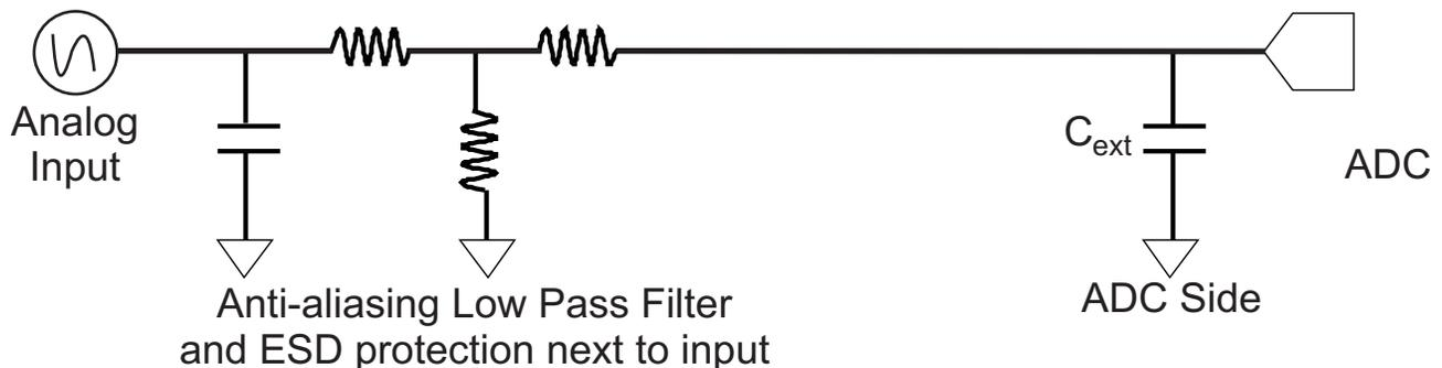
Figure 8. ADC Input Passive Circuit (No OP\_AMP)
