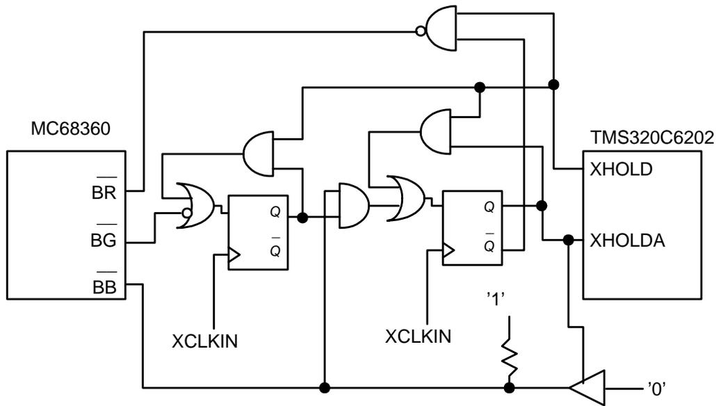
**Figure 2. Block Diagram of External Bus Arbiter Used in Interface Between MC68360 (Host) and C6000 Expansion Bus**
