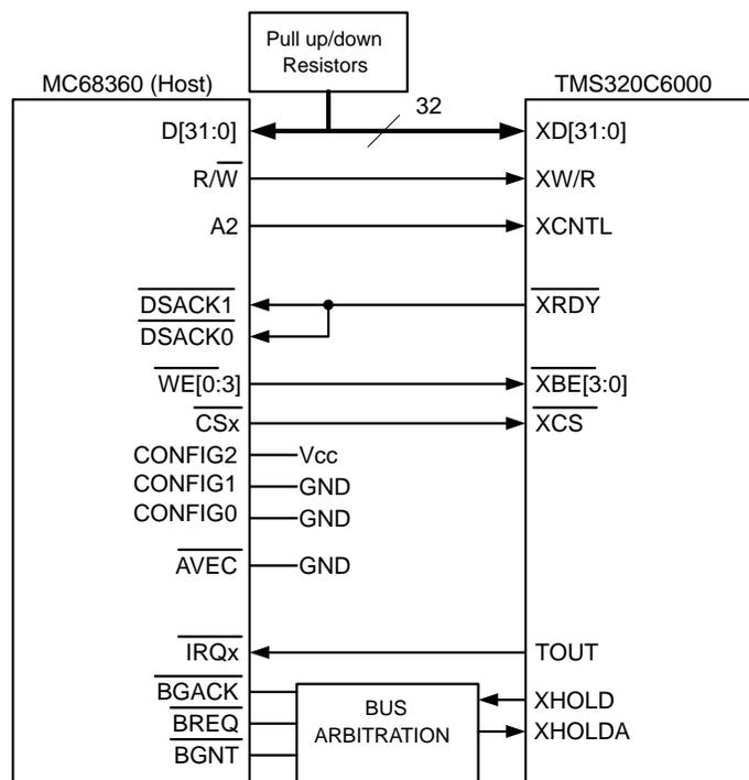
**Figure 1. Block Diagram of Interface Between MC68360 (Host) and Expansion Bus**
