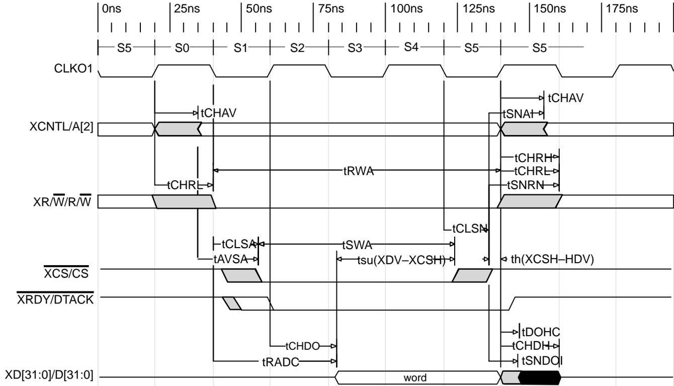
Figure 4. MC68360 (Host) Performs Write to Expansion Bus Interface
