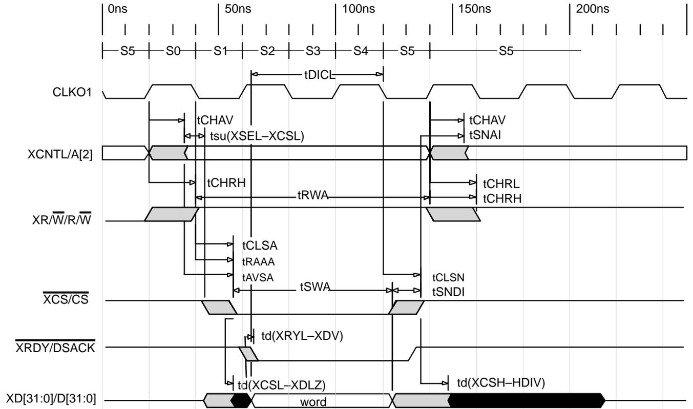
**Figure 3. MC68360 (Host) Performs Read from Expansion Bus Asynchronous Host Port Interface**
