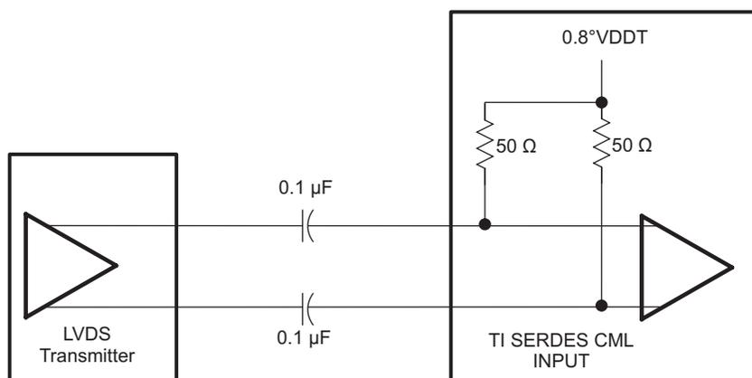
**Figure 1. LVDS to CML Connection Basic Diagram**
