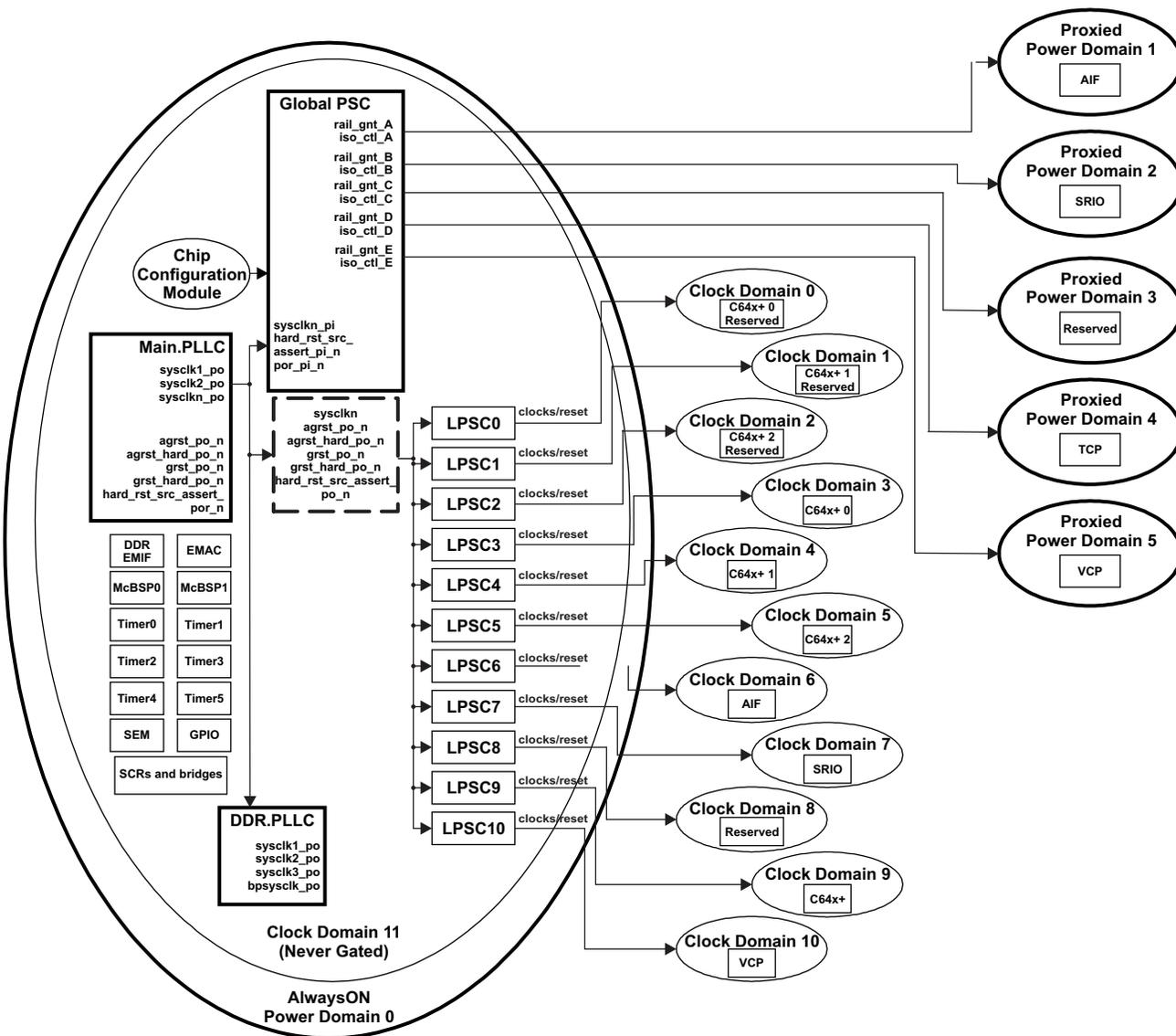
Figure 1 shows all of the power and clock domains on the device. As shown, many modules reside in the AlwaysOn domain, which always has power and clocks provided. These consist primarily of the infrastructure components that are responsible for the clock and reset control (PLL Controller, PSC), the switch fabric that connects all of the modules, and small modules that don't need dynamic enable/disable because they do not consume a significant amount of power.
