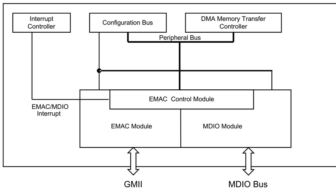
Figure 1 shows the main interface between the EMAC control module and the CPU. The following connections are made to the device core:
