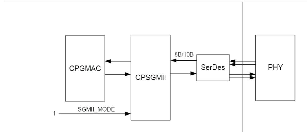
The following setup shows the CPSGMII setup for this mode of operation:
