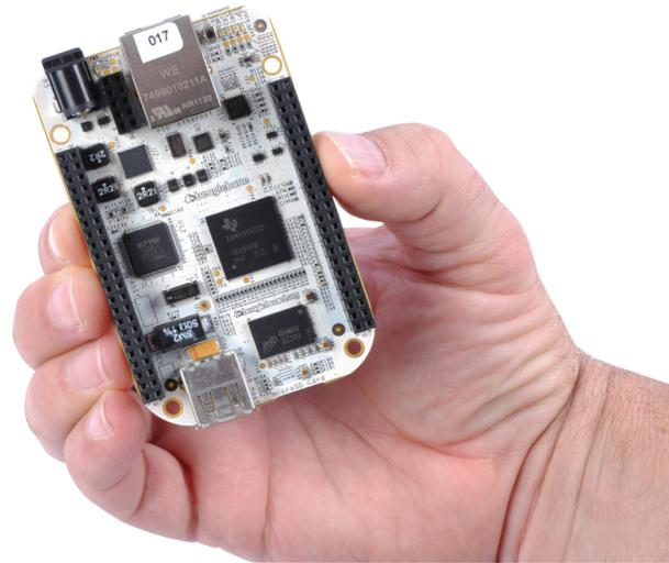
To accommodate a range of sensors, controls, and other types of inputs, it has two 46-pin expansion headers featuring 66 general purpose interrupt generating input/output (GPIO) pins at 3.3V and multiplexed with LCD signals, a parallel memory bus, secondary MMC/SD/SDIO
