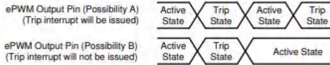
**Workaround(s):** Avoid configuration of blanking window such that the trip input would fall in this range (1 cycle before and 3 cycles after the blanking window closure).
