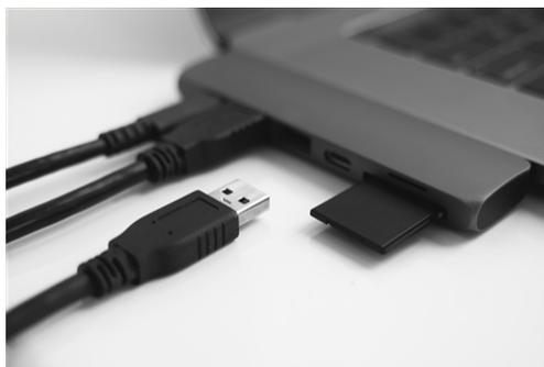
**Figure 1. Example laptop docking station with USB PD**
