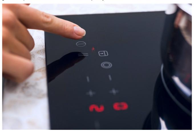
Figure 1. Cooktop Controls Using Capacitive Touch
