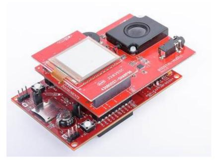
Figure 2. Filtering and signal processing reference design
