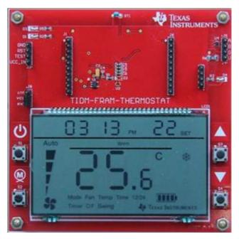
Figure 1. Example of thermostat implementation with FRAM MCUs reference design
