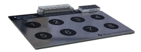
Figure 3. CapTlvate technology access control panel
