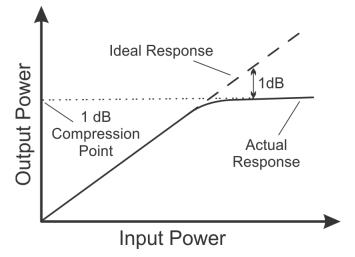
Figure 2. Output P1dB Example
