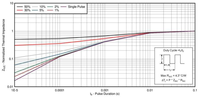
Figure 1. CSD17579Q5A Normalized Transient Thermal Impedance Curve
