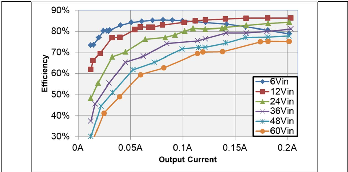
Figure 1 Efficiency vs Output Current
