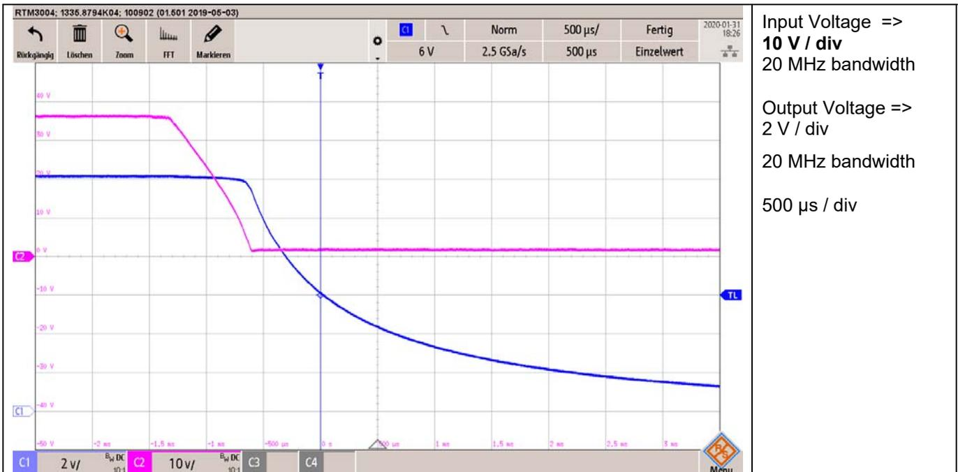
Figure 27 Shut-down @ 36 V Input Voltage
