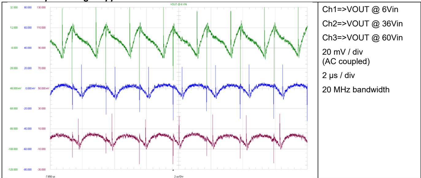
**Figure 15 VOUT @ 6 V Input Voltage**
