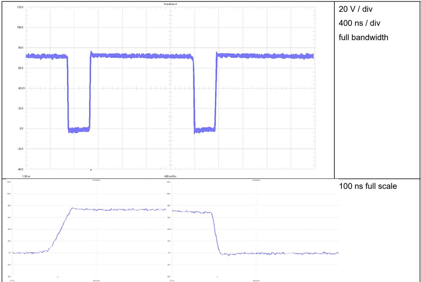
**Figure 11 SW-to GND @ 60 V Input Voltage**
