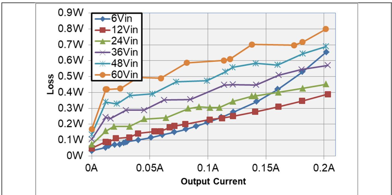
Figure 2 Loss vs Output Current
