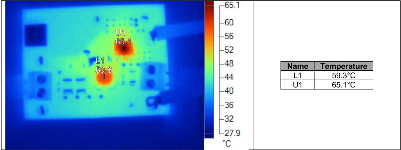
**Figure 8 Thermal Image at 60 V Input Voltage**
