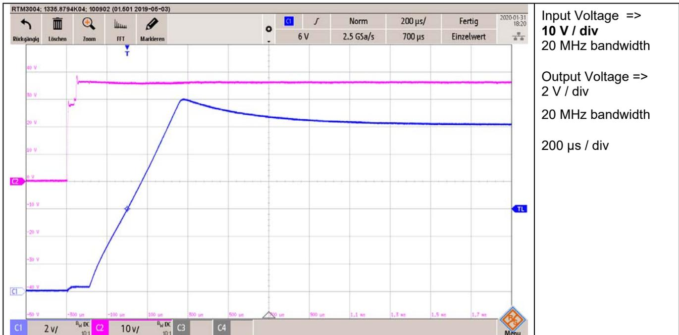
Figure 24 Start-up @ 36 V Input Voltage
