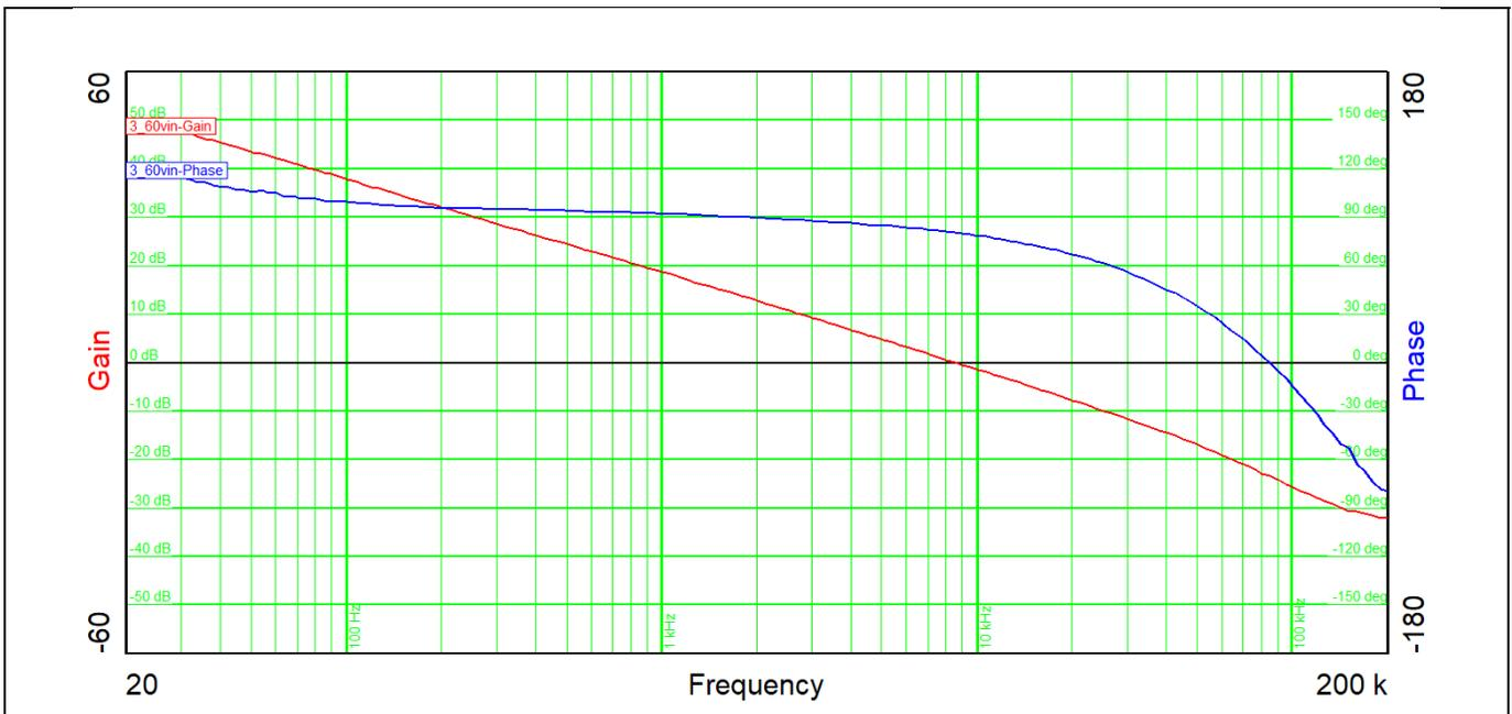
Figure 19 Frequency Response for 60 V Input Voltage
