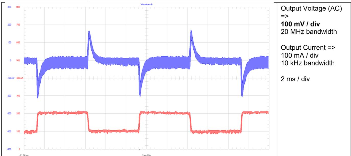
**Figure 21 Load Transient for 36 V Input Voltage**
