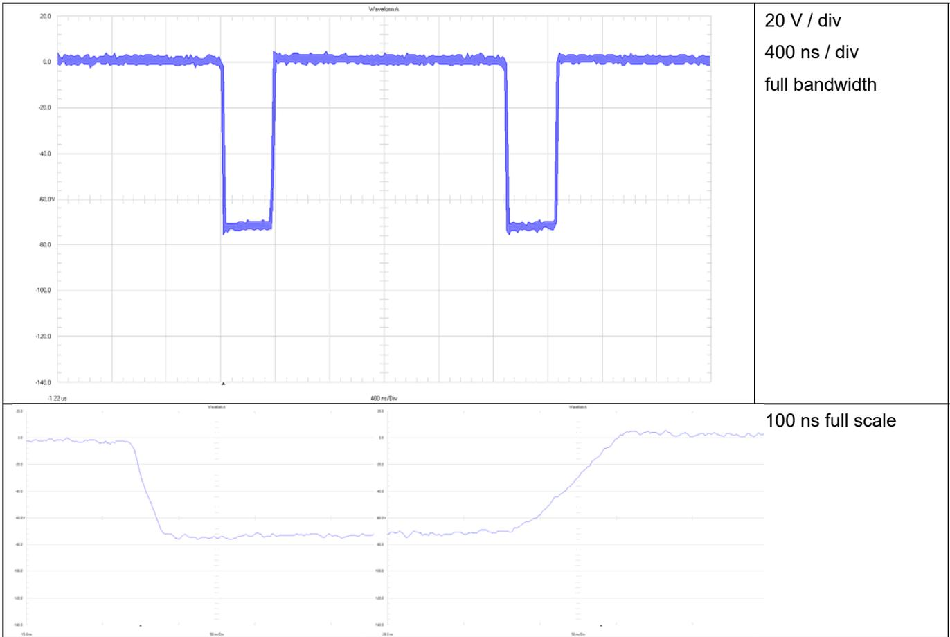
**Figure 14 D1 @ 60 V Input Voltage**
