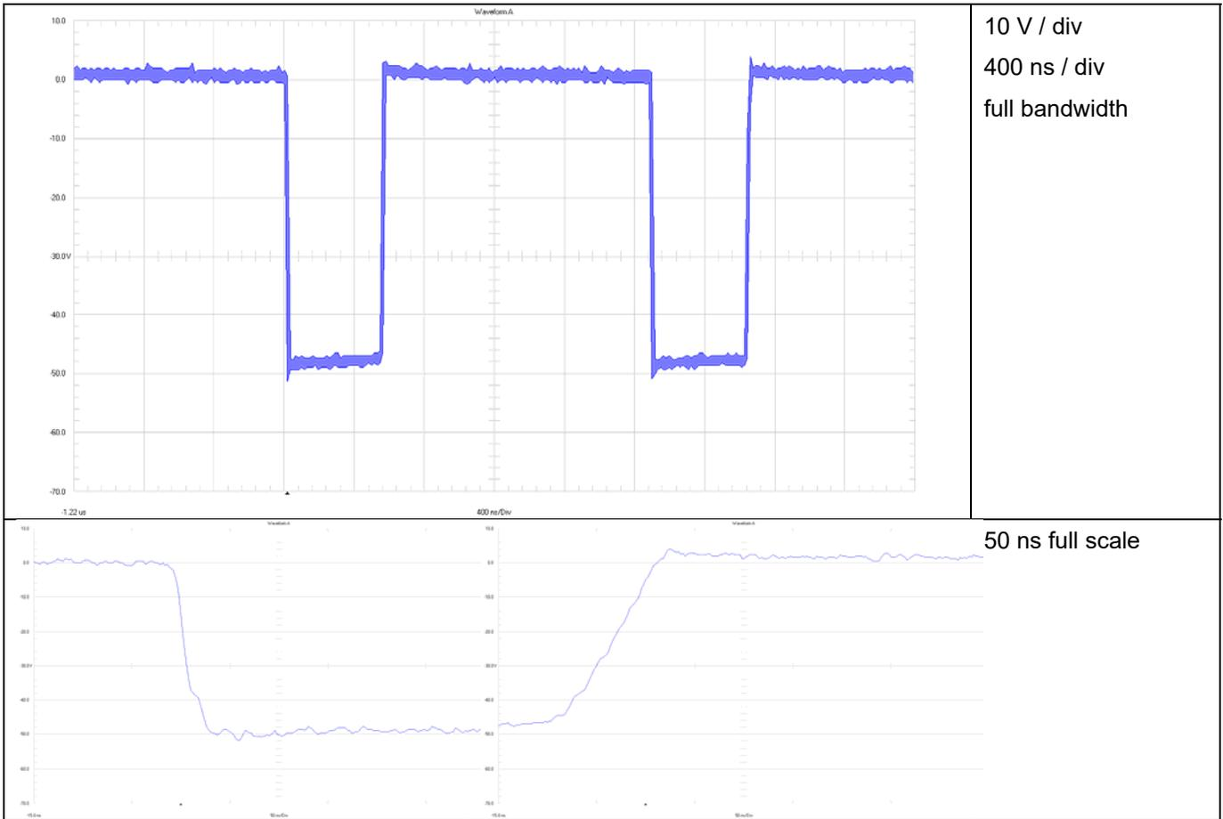
**Figure 13 D1 @ 36 V Input Voltage**
