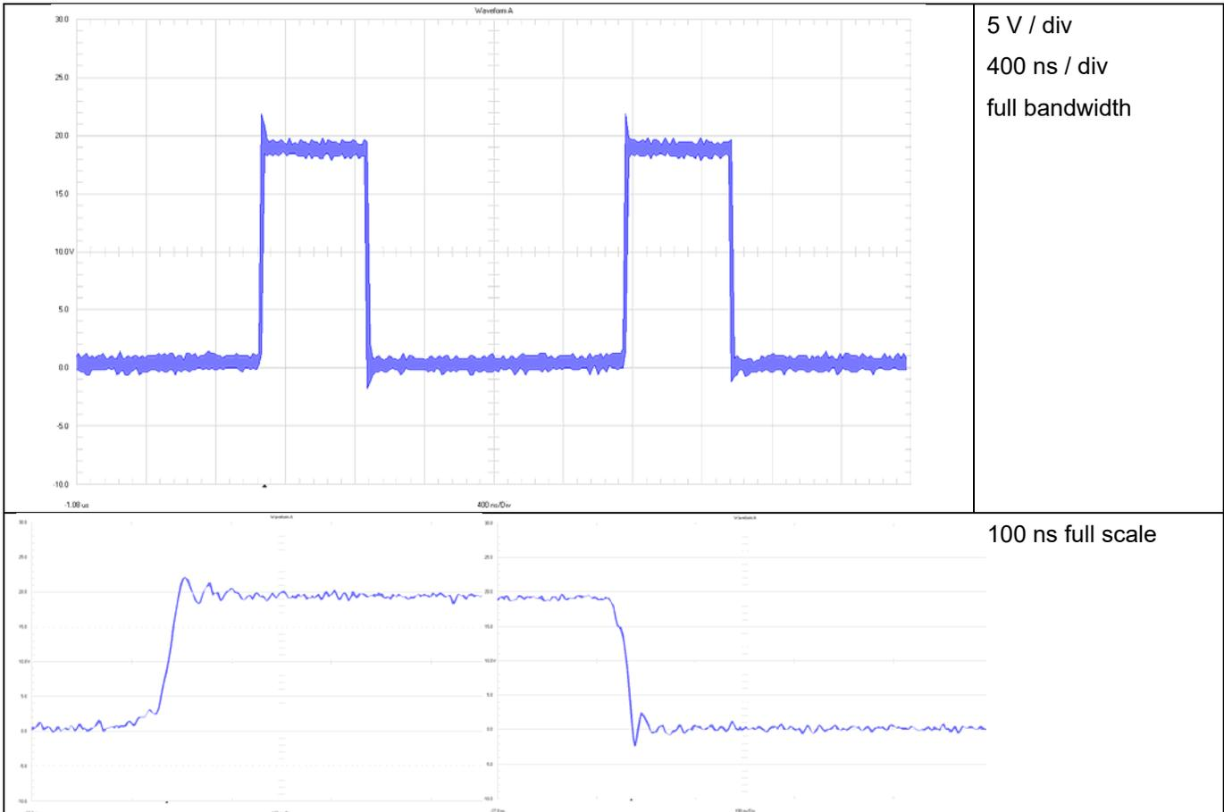
**Figure 9 SW-to GND @ 6 V Input Voltage**
