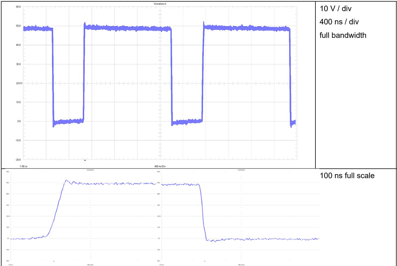
Figure 10 SW-to GND @ 36 V Input Voltage
