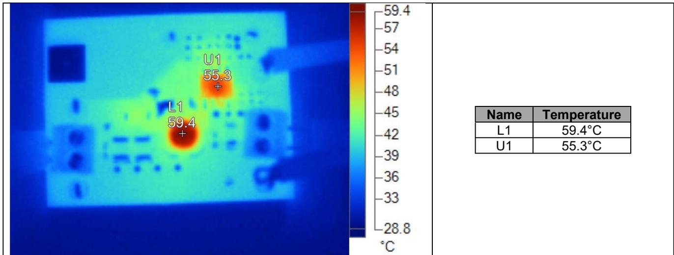
Figure 6 Thermal Image at 6 V Input Voltage
