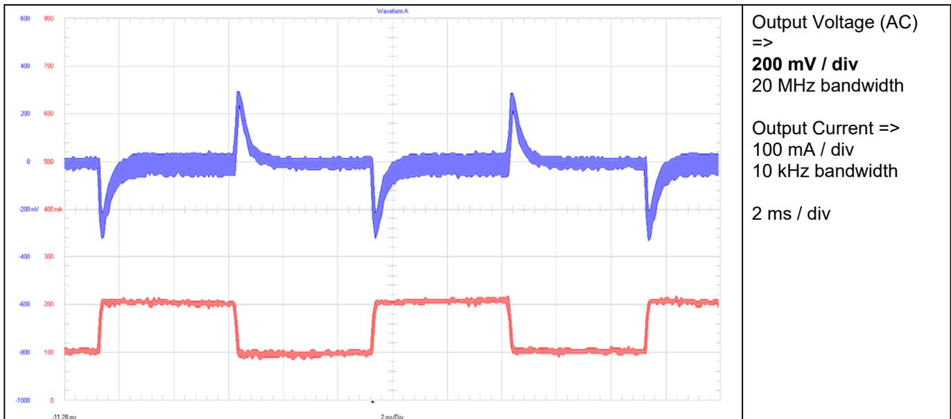
**Figure 20 Load Transient for 6 V Input Voltage**
