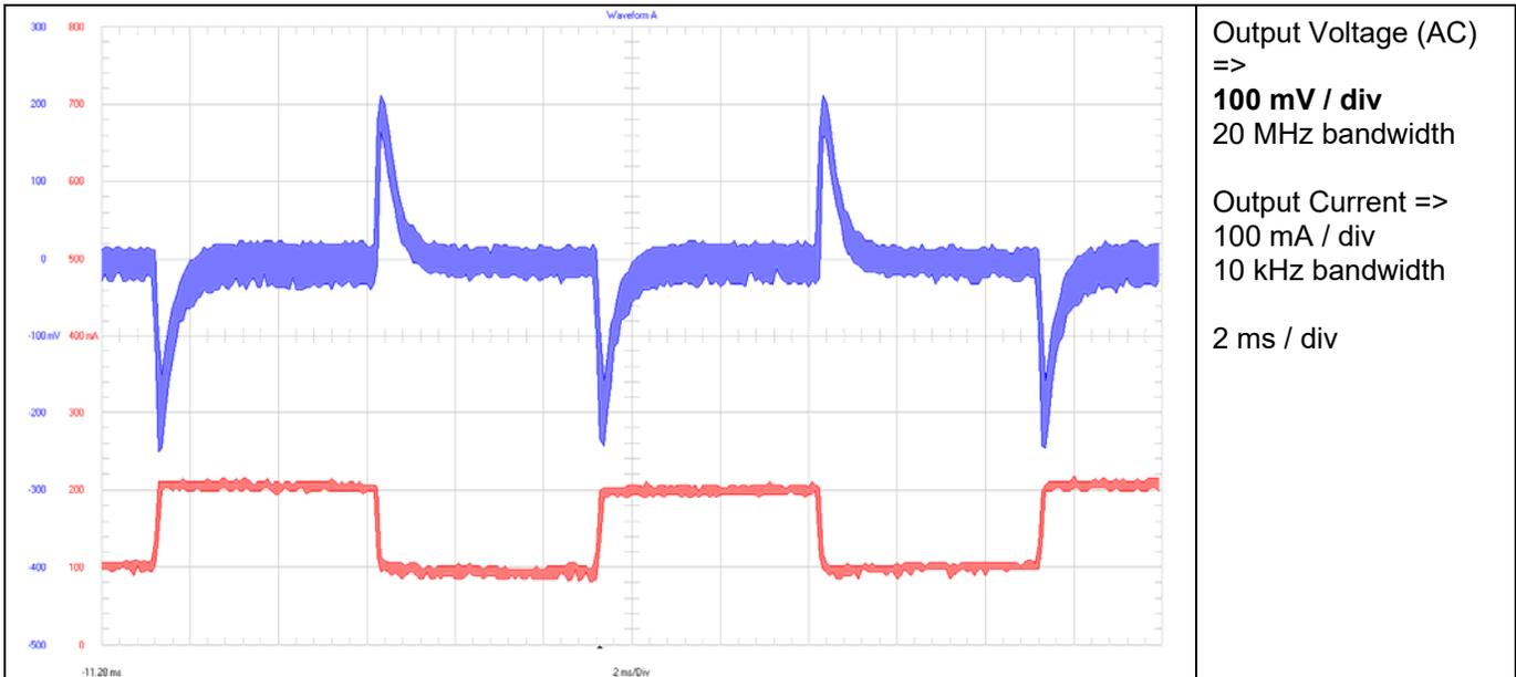
**Figure 22 Load Transient for 60 V Input Voltage**
