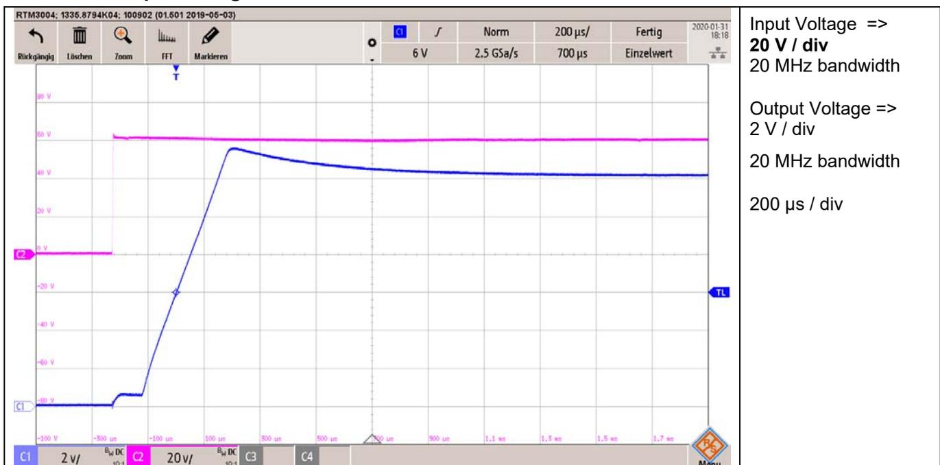
Figure 25 Start-up @ 60 V Input Voltage
