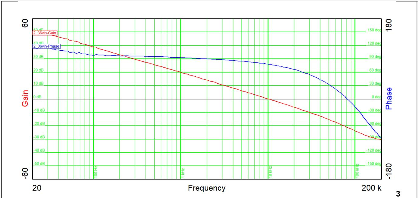
Figure 18 Frequency Response for 36 V Input Voltage
