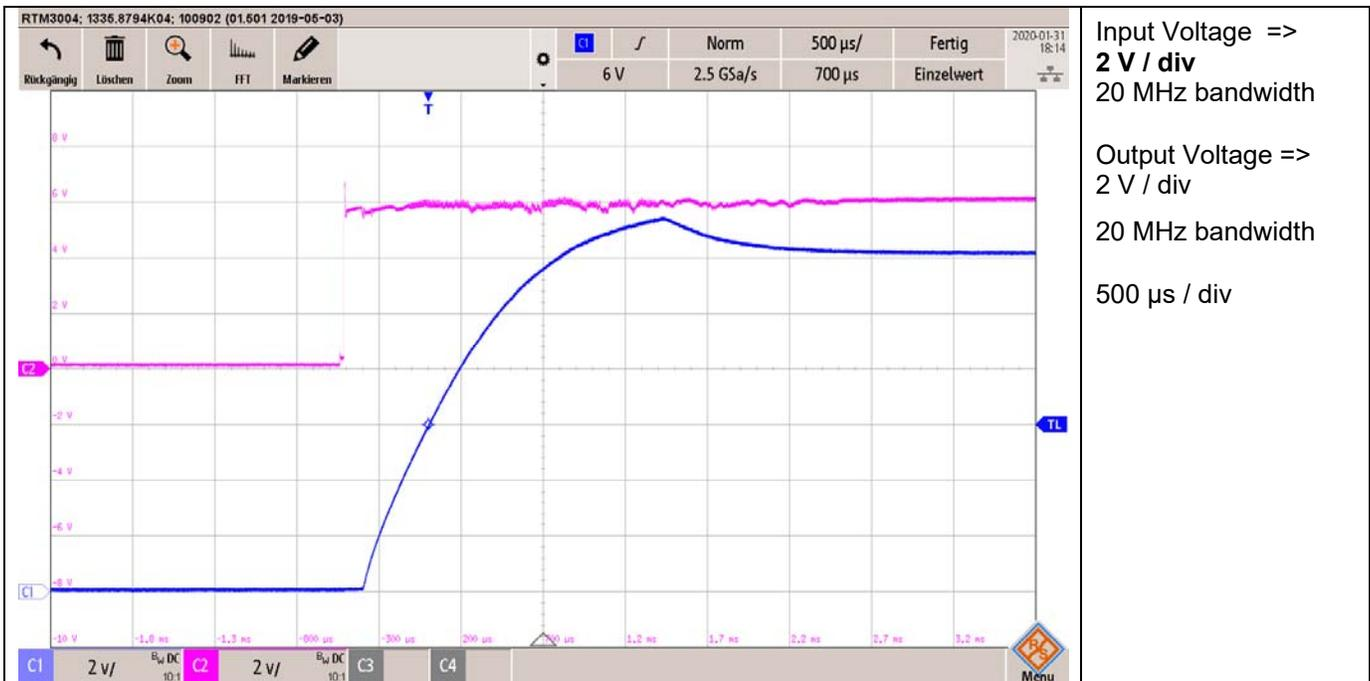
**Figure 23 Start-up @ 6 V Input Voltage**
