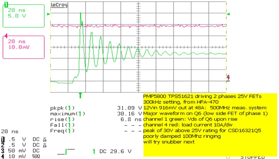
Such waveforms will have both System EMC Engineer and Reliability Engineer screaming !!!
