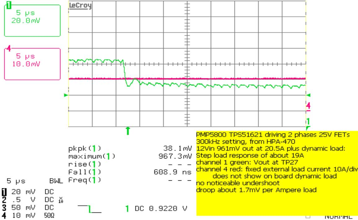
Load dump response using same on board dynamic load:
