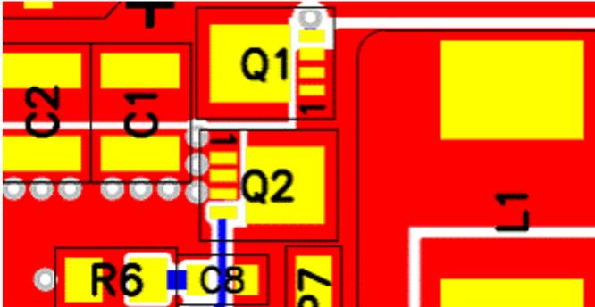
Q1 is the high side FET; Q2 is the low side FET; C1 and C2 are the input caps (ceramic size 1210); C8 and R6 is the snubber. Key is rotating Q1 and Q2 such that drain of high side FET and source of low side FET face same side where the input caps are to be placed. Snubber then should be placed as close to drain source of low side FET as feasible. Traces to gates are much less critical and can be on other layers and be signal trace (10 to 25 mils) width.
