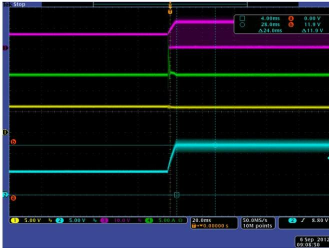
Start up Full Load, With UVLO Used as enable.
