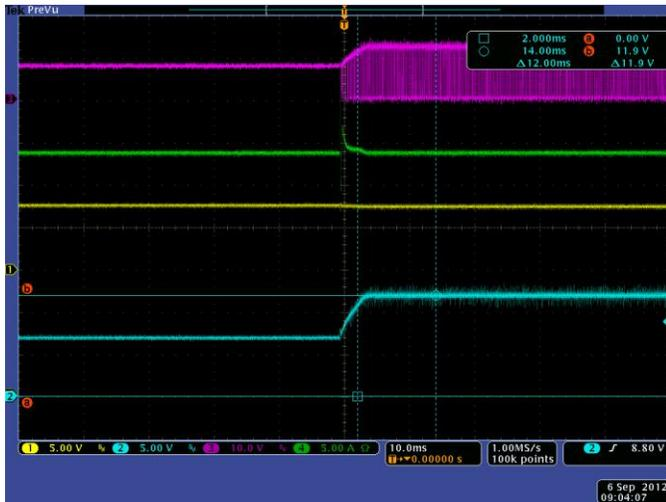
Start Up Full Load, 8V in With UVLO Used as enable. Ch 1 Vin, Ch 2 Vout, Ch 3 Vswitch, Ch 4 Iin
