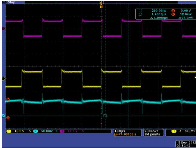
Ch2 2, Master Inductor Current – 34A out (Measured across 1.5mR current sense Resistor)
