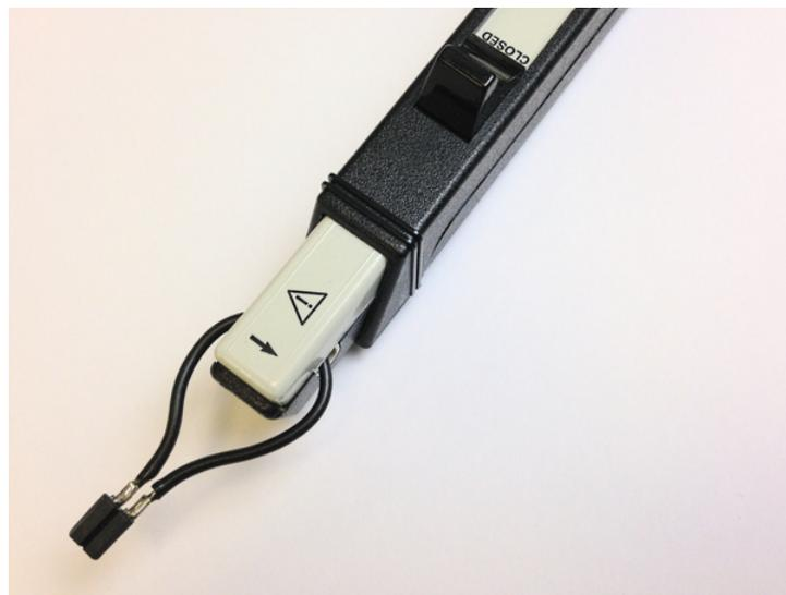
Figure 23. Combination of Current Probe With Self-Made Adapter for Primary Side Current Measurement
