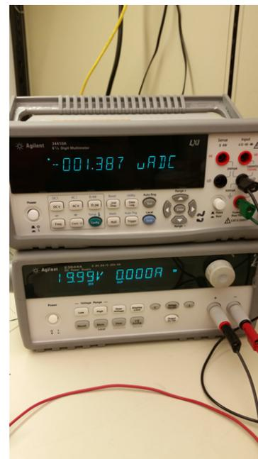
Figure 29. Reverse Polarity Measurement With Inverted Polarity
