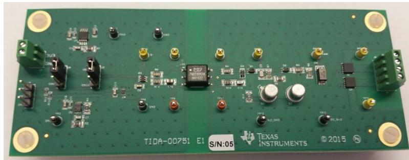
**Figure 14. TIDA-00751 Reference Design Hardware**
