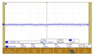
Figure 3-8. Output Voltage Ripple - 1.8 V
