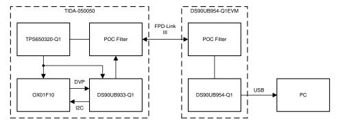
Figure 3-3. Block Diagram of Characterization Test Setup
