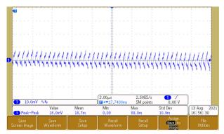
Figure 3-6. Output Voltage Ripple - 3.8 V
