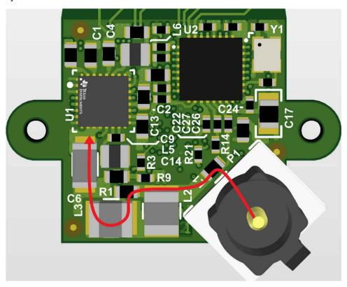
Figure 4-1. PCB Layout With POC Routing
