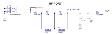
Figure 1-1. FPD-Link III Signal Path
