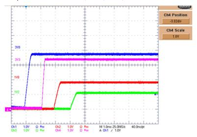
(Channel 1): 3.3-V supply; (Channel 2): 2.9-V supply; (Channel 3): 1.2-V supply; (Channel 4): 1.8-V supply
