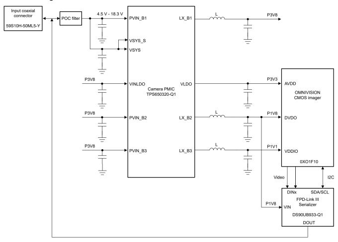
Figure 2-1. Camera Block Diagram
