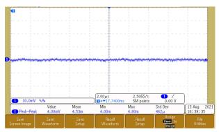
Figure 3-7. Output Voltage Ripple - 3.3 V
