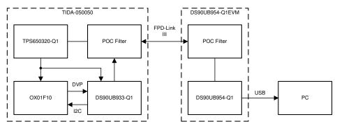
Figure 3-2. Block Diagram of Test Setup
