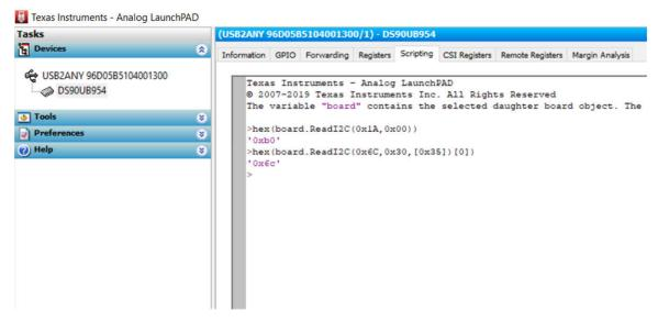
Figure 3-12. Back-Channel I2C Communication
