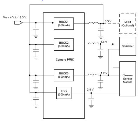
Figure 2-5. TPS650320-Q1 Typical Application Circuit
