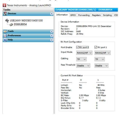
Figure 3-10. Analog LaunchPad™ Link Confirmation
