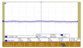
Figure 3-9. Output Voltage Ripple - 1.1 V
