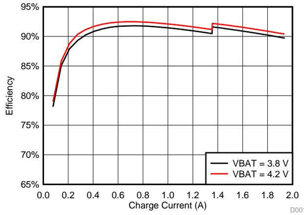
Figure 3. Charging Efficiency at VBUS = 5 V
