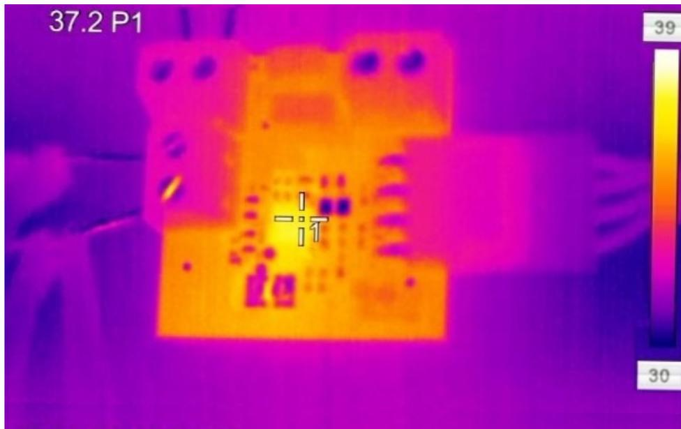
Figure 4. Thermal Performance at VBUS = 5 V and ICHG = 0.5 A
