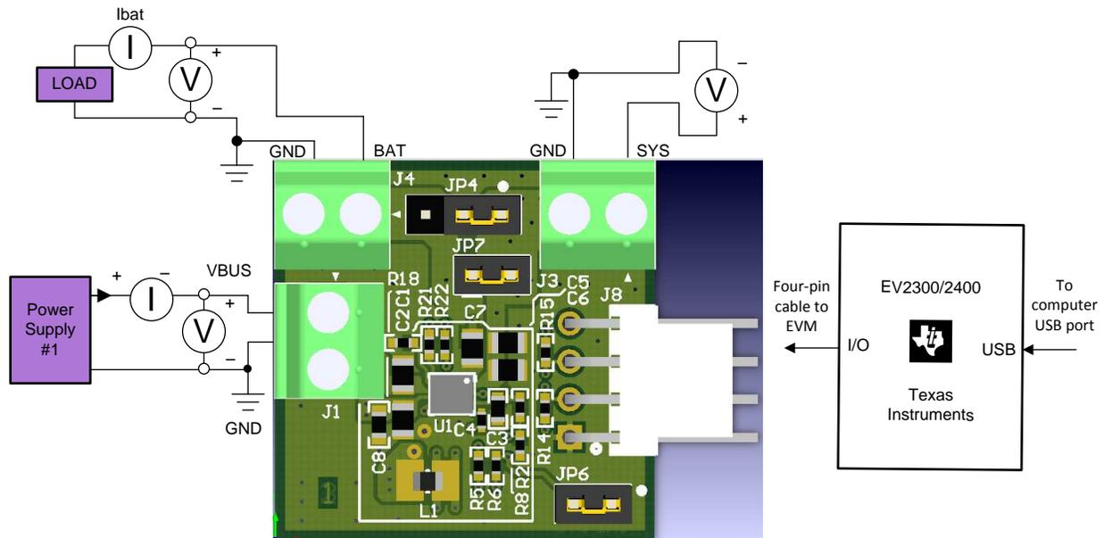
Figure 2. Test Setup
