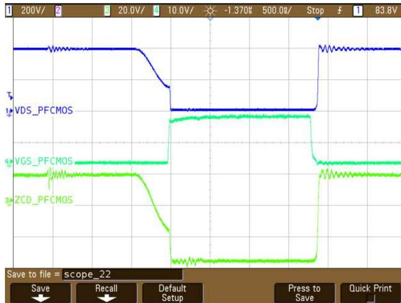
Figure 12. PFC MOSFET Switching Waveform
