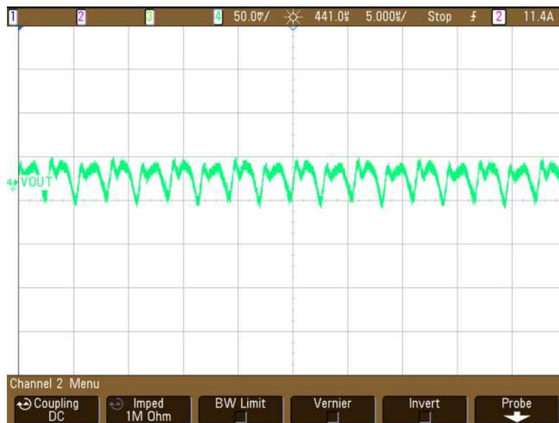
Figure 10. Output Voltage Ripple at Full Load
