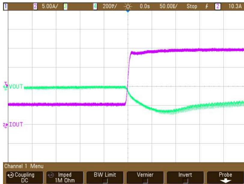
Figure 9. Load Transient Response
