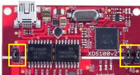
**Figure 13. F28379D Jumper Configuration**
