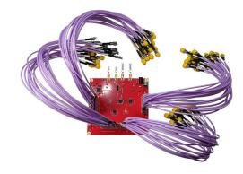
Cascaded Clock Distribution Reference Design Supports 16 High Frequency Outputs 1
