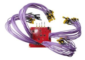
Figure 3-2. Cascaded Clock Distribution Board with RF Cables
