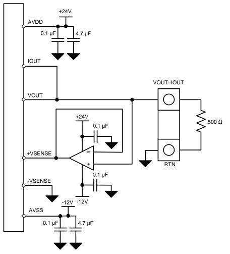
Figure 13. Bipolar Supply Connections for the +VSENSE Buffer
