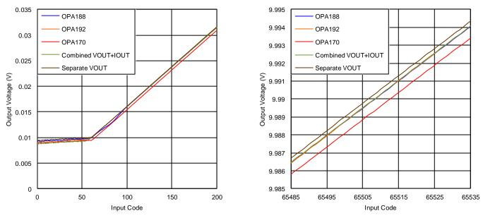
Figure 12. 0-V to 10-V Output Results with Unipolar Supplies
