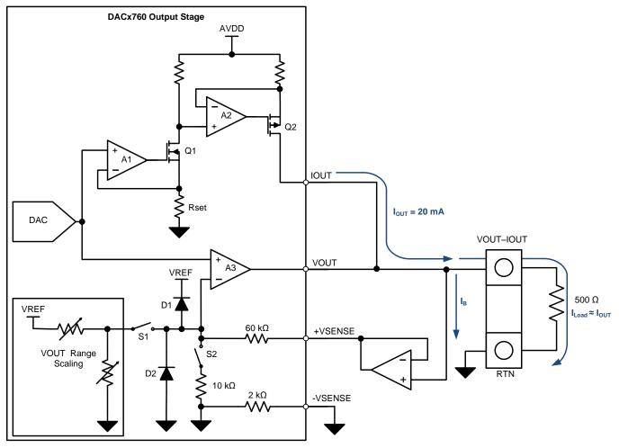
Figure 9. Buffering the +VSENSE Pin Using an External Amplifier
