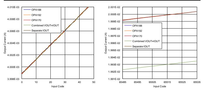
Figure 11. 4-mA to 20-mA Output Results with Unipolar Supplies
