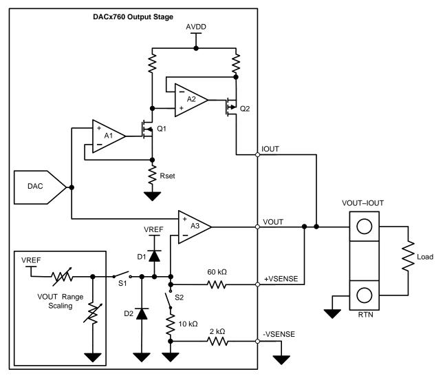
Figure 2. Combining the Voltage and Current Output Circuits
