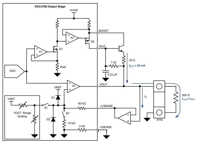
Figure 16. Buffering the +VSENSE Pin Using an External Amplifier with a Boost Transistor
