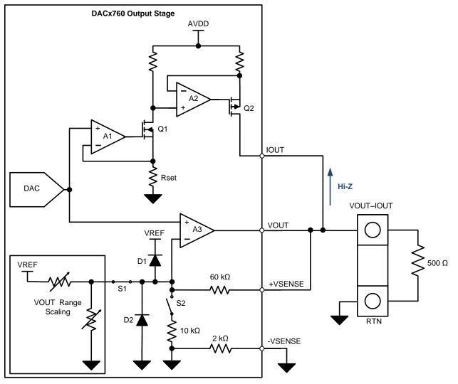
Figure 3. Voltage Mode Operation with a Combined VOUT-IOUT Connection
