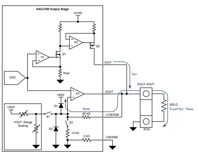
Figure 4. Current Mode Operation with a Combined VOUT-IOUT Connection
