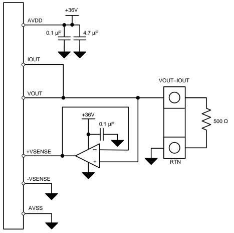
Figure 10. Unipolar Supply Connections for the +VSENSE Buffer
